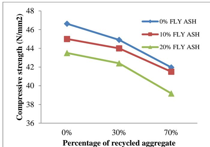
Figure 2: Variation of Cubes Compressive Strength Results
