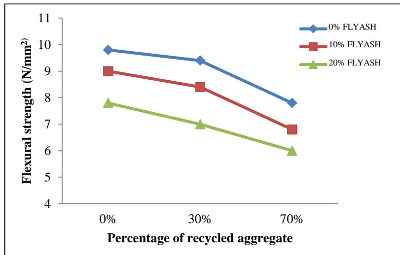
**Figure 5: Variation of Flexural Strength Test Results**
