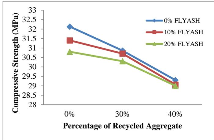
Figure 1: Variation of Cubes Compressive Strength Results
