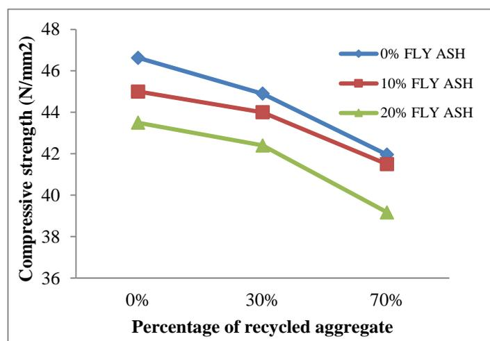
**Figure 3: Variation of Cylinder Compressive Strength Results with replacement by recycled Aggregates**
