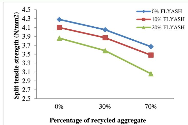
**Figure 4: Variation of Cylinder Split Tensile Strength Results**
