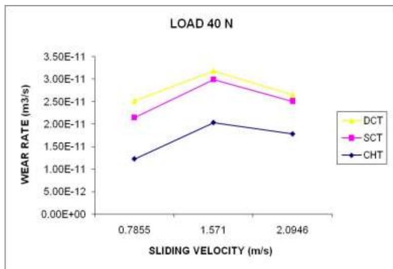
Figure 2 Wear Rate at 40 N for Three Different Treatments
