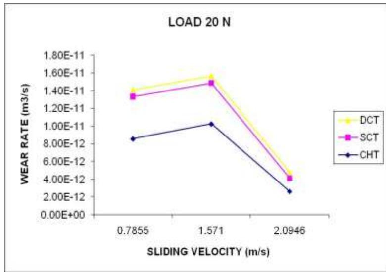
Figure 1 Wear Rate at 20 N for Three Different Treatments
