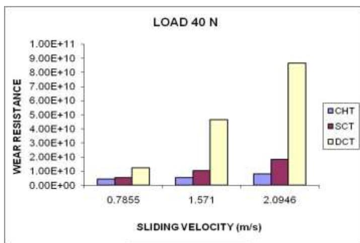
Figure 4 Wear Resistances at 40 N for Three Different Treatments
