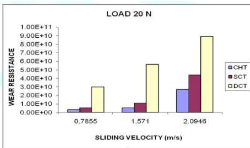
Figure 3 Wear Resistances at 20 N For Three Different Treatment
