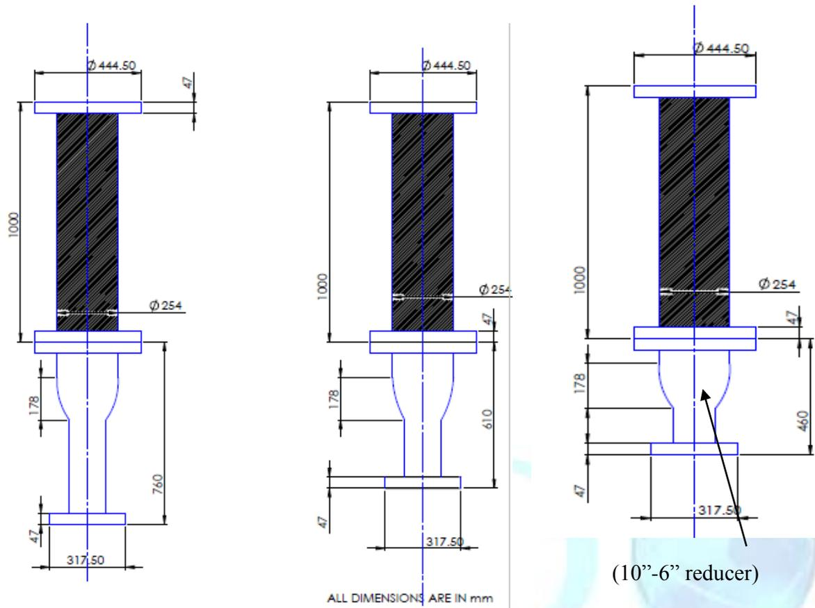
Fig 3. Bellows connected with spools
