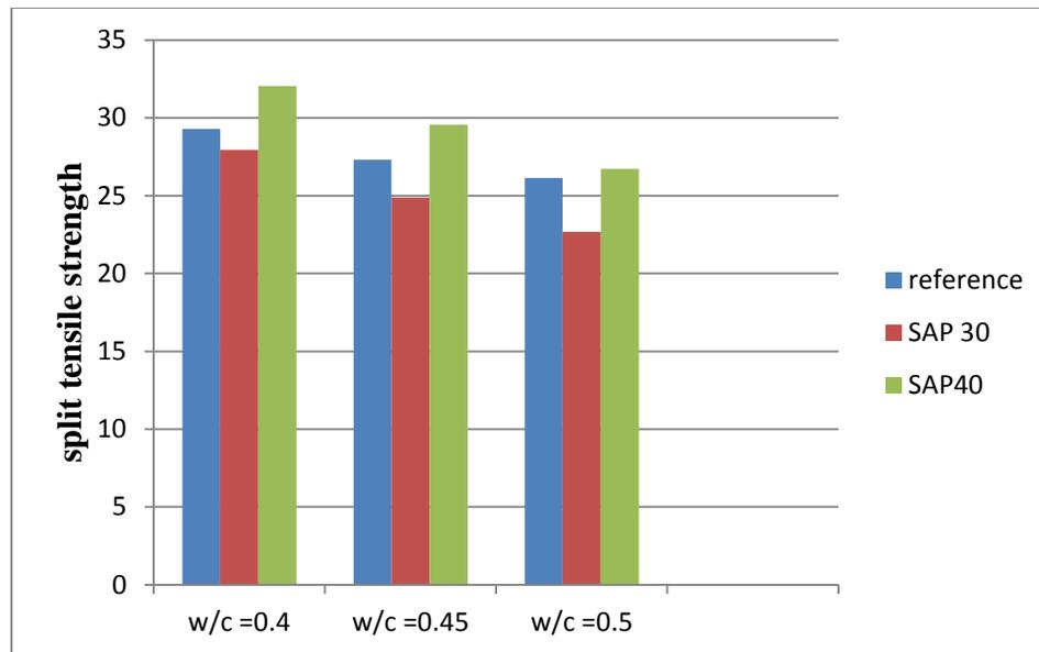
Figure 3 :7 Days Split Tensile Strength (N/Mm<sup>2</sup>)
