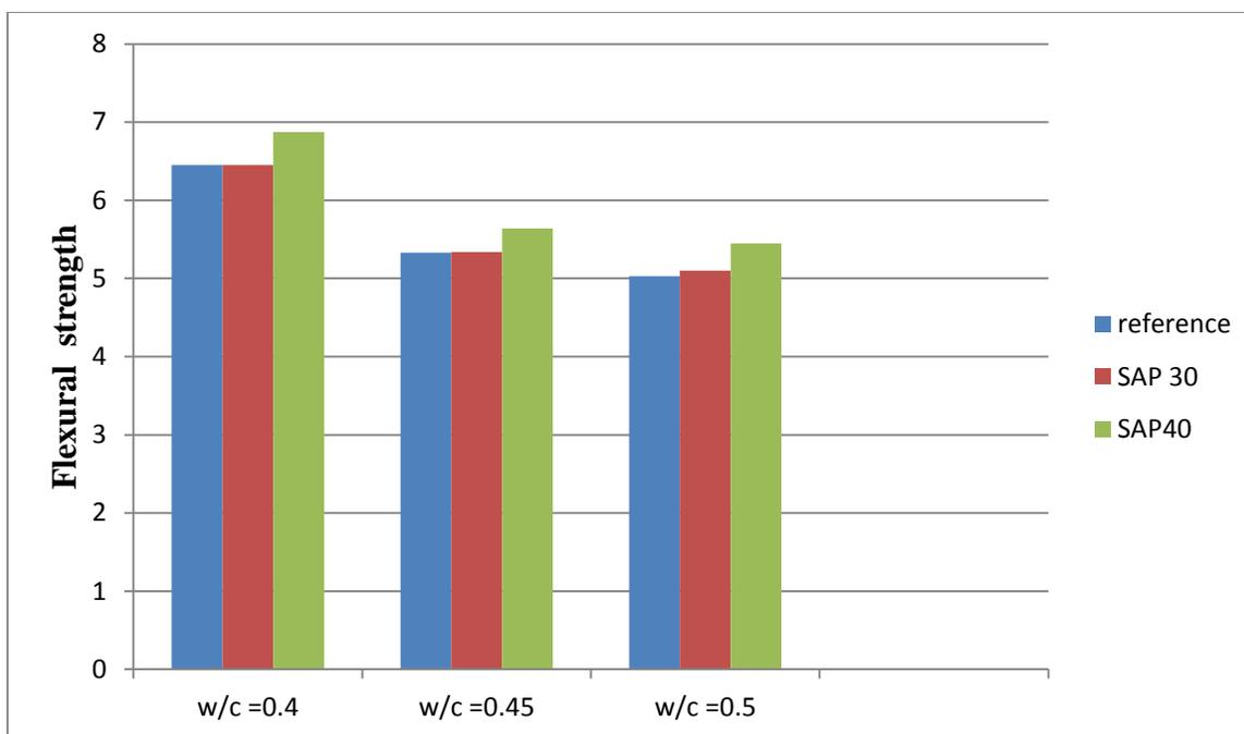
Figure6: Flexural Strength (28 Days)
