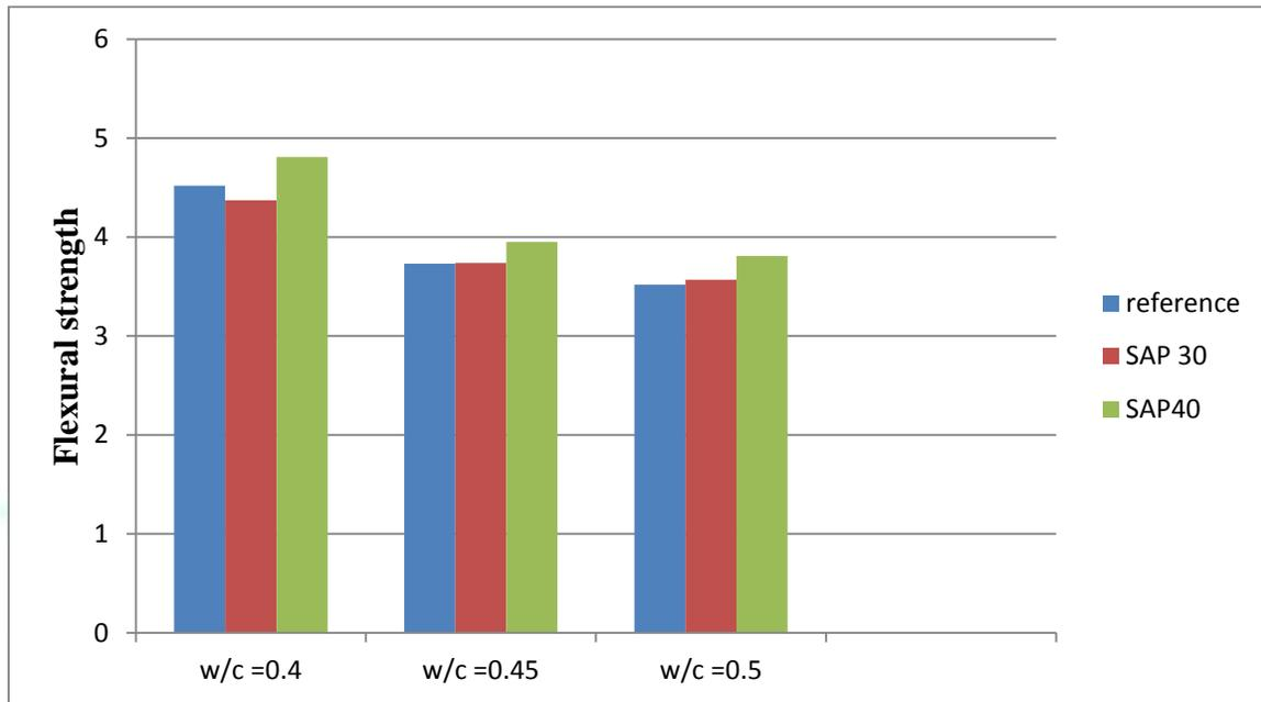
Figure5 : Flexural Strength (7 Days)
