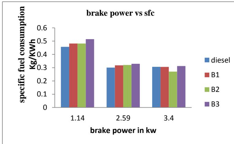
Graph .2: specific fuel consumption Vs brake power of a diesel and its blends
