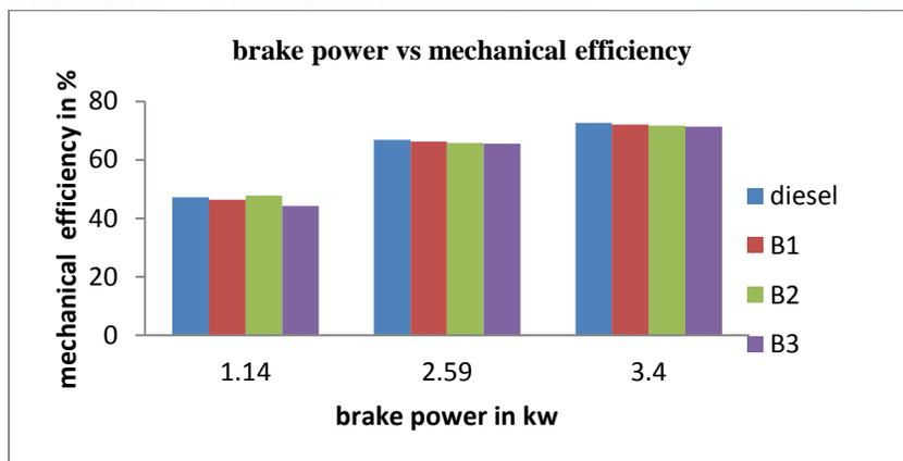
Graph 4: mechanical efficiency Vs brake power of a diesel and its blends.
