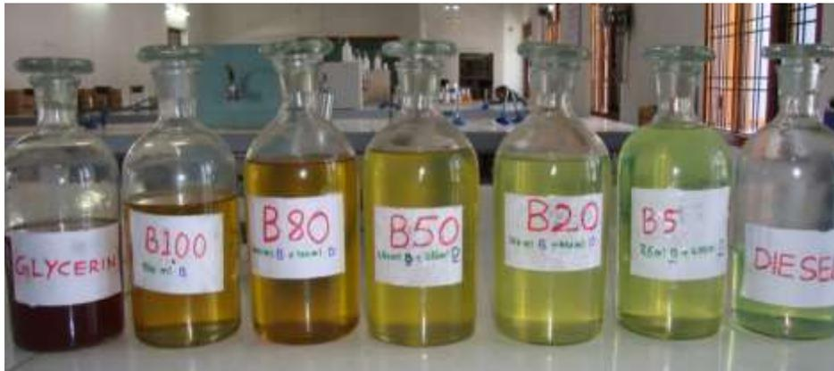
Fig 1: prepared samples of bio diesel blends and diesel
