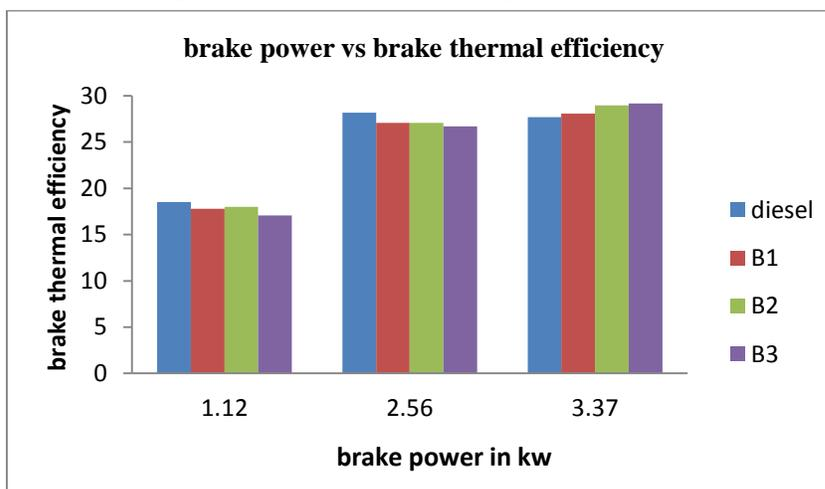
Graph 3: Brake thermal efficiency Vs brake power of a diesel and its blends.
