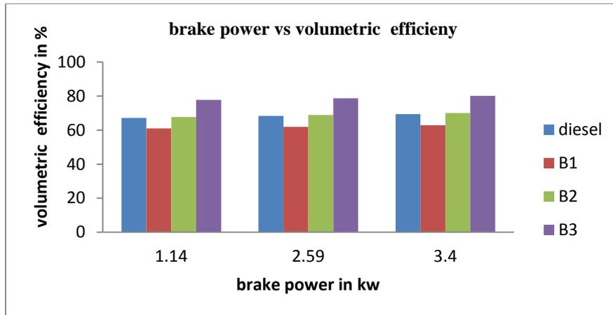
Graph 5: volumetric efficiency Vs brake power of a diesel and its blends.
