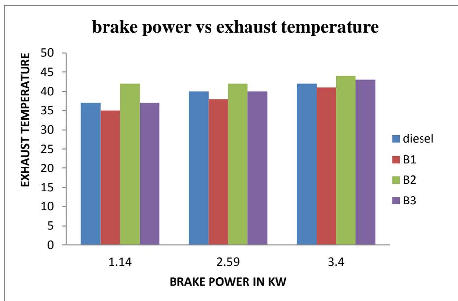
Graph 6: exhaust temperature Vs brake power of a diesel blends.
