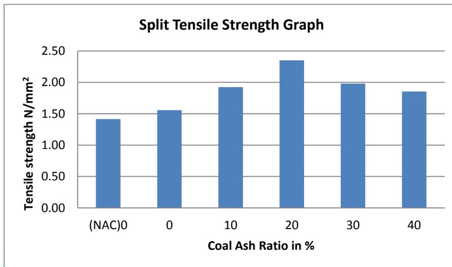
**Figure 3. Graph result for Split tensile strength at 28 days**
