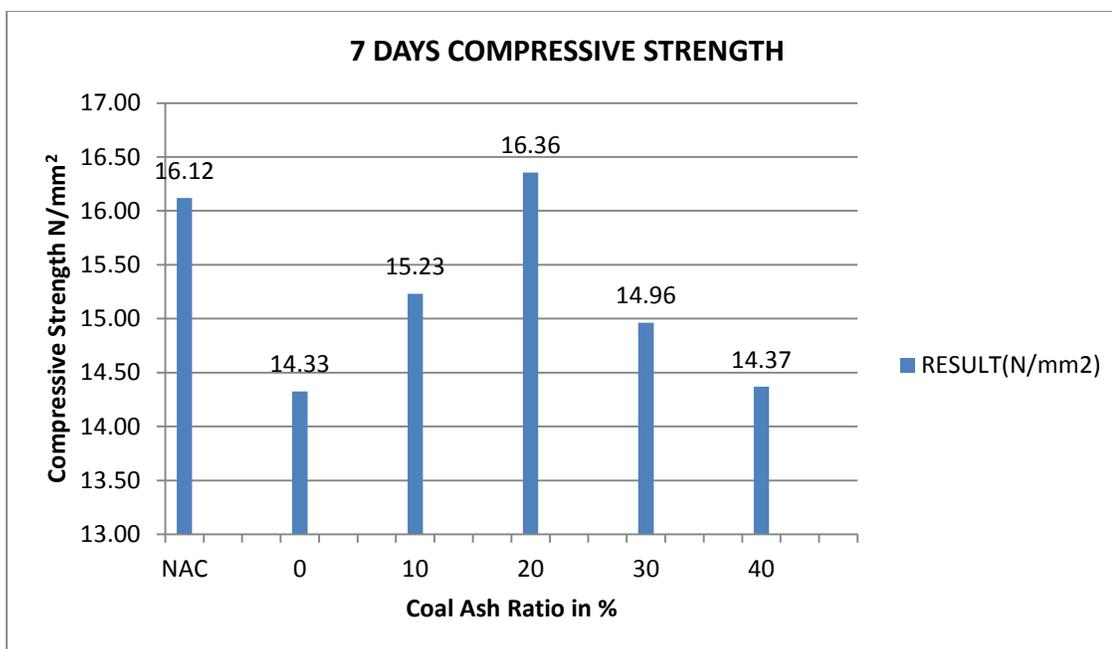
Figure 1. Graph result for compressive strength at 7 days
