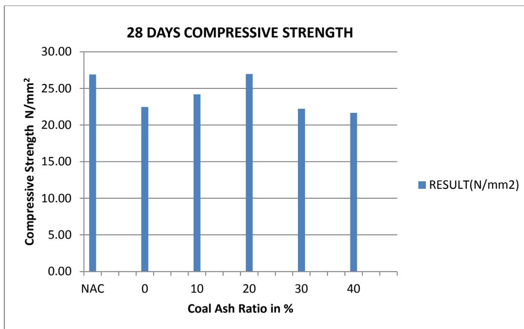
Figure 2. Graph result for compressive strength at 28 days
