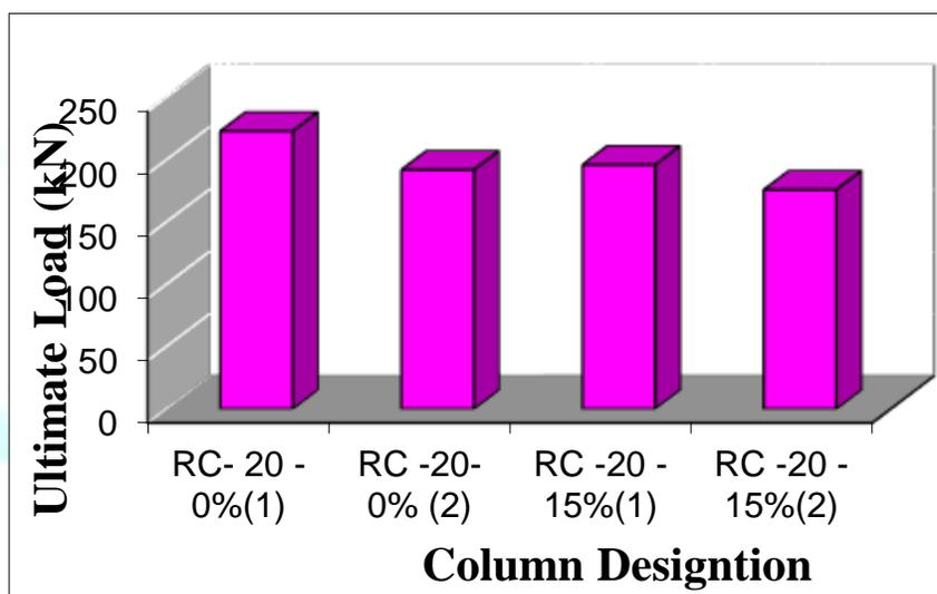
**Figure 2.**Compressive strength of all columns with M20 grade-comparison
