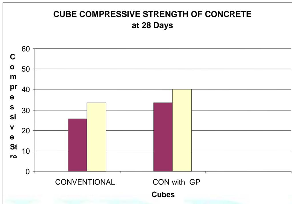
**Figure 1: Average Compressive Strength Of Cube At 28 Days**
