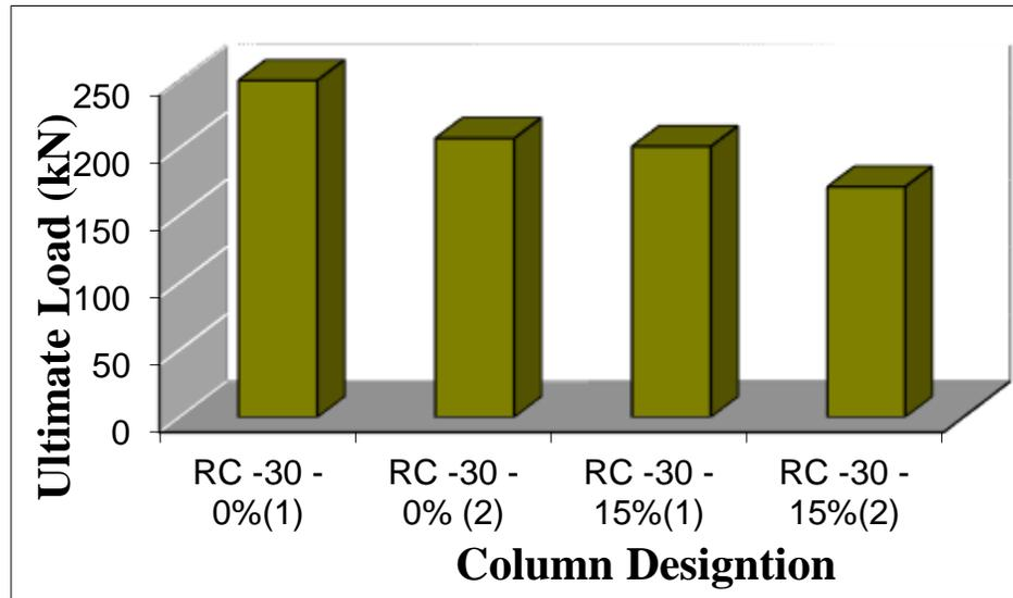
Figure 3.Compressive strength of all columns with M30 grade-comparison
