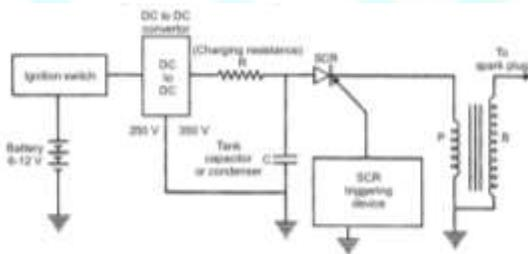
Depending upon the engine firing order, whenever the SCR triggering device, sends a pulse, then the current flowing through the primary winding is stopped. And the magnetic field begins to collapse. This collapsing magnetic field will induce or step up high voltage current in the secondary, which while jumping the spark plug gap produces the spark, and the charge of air fuel mixture is ignited.
