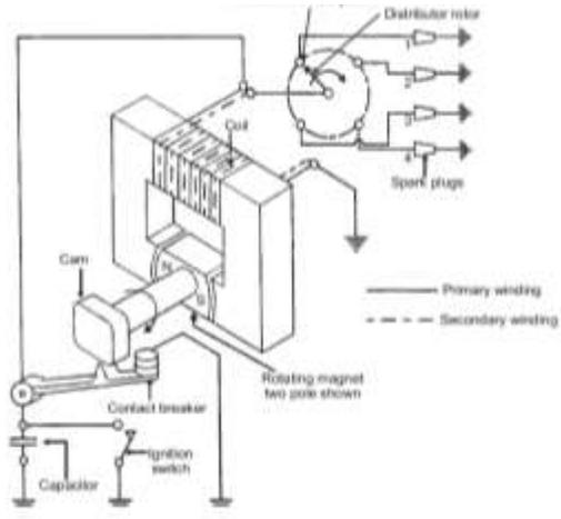
**Figure : Schematic Diagram of Coil/Battery Ignition System**
