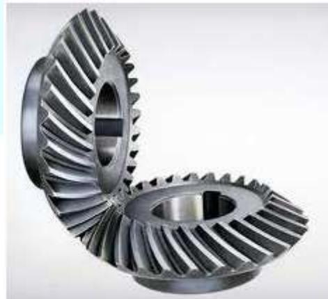
Zero Bevel gear: Zero Bevel gears are similar to straight bevel gears, but their teeth are curved lengthwise. These curved teeth of zero bevel gears are arranged in a manner that the effective spiral angle is zero.
