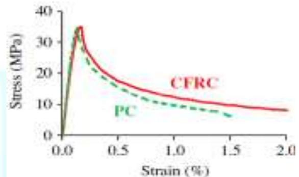
**Fig: 2 Stress v/s strain graph for CFRC & PC. (Source: Google)**
