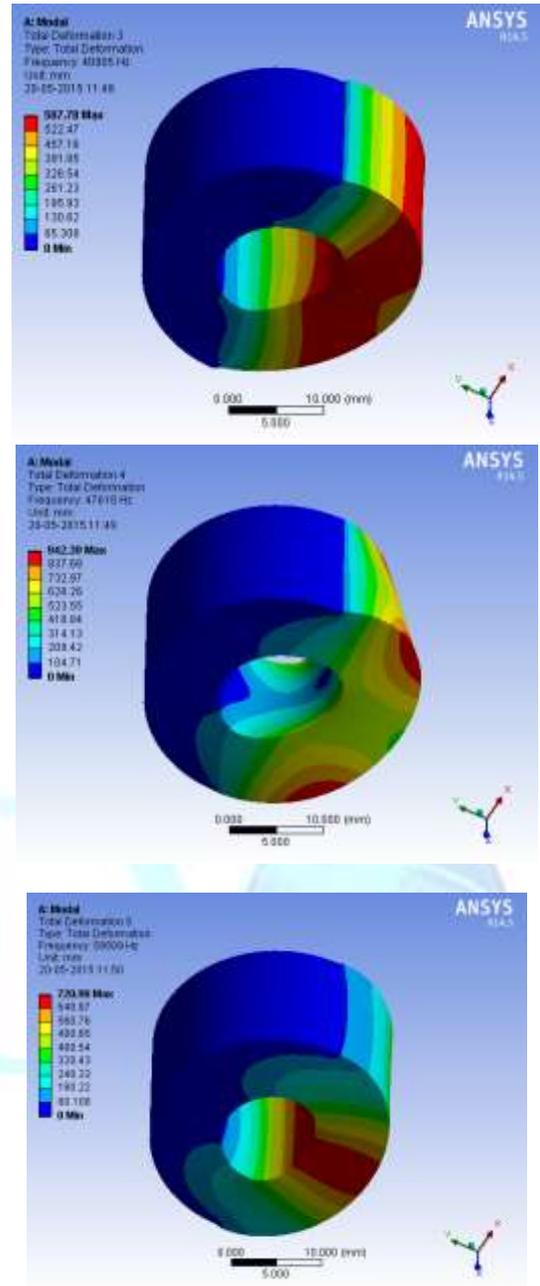
Fig 2.4 : Modal frequency at mode number 1,2,3,4,5, for Cast Nylon bush
