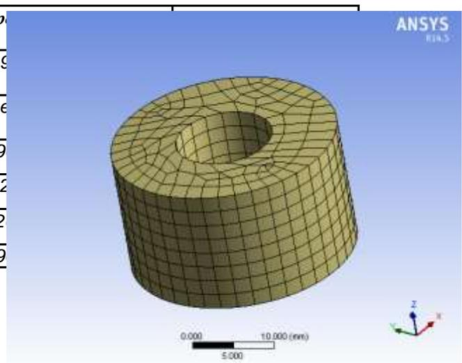
Fig 2.3 : Meshing of Bearing
