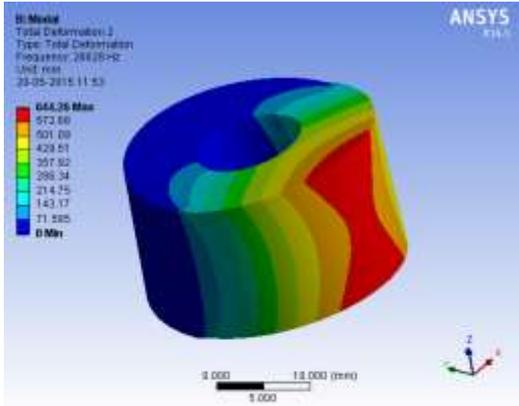
Fig 2.5 : Modal frequency at mode number 1,2,3,4,5, for Epoxy glass bearing
