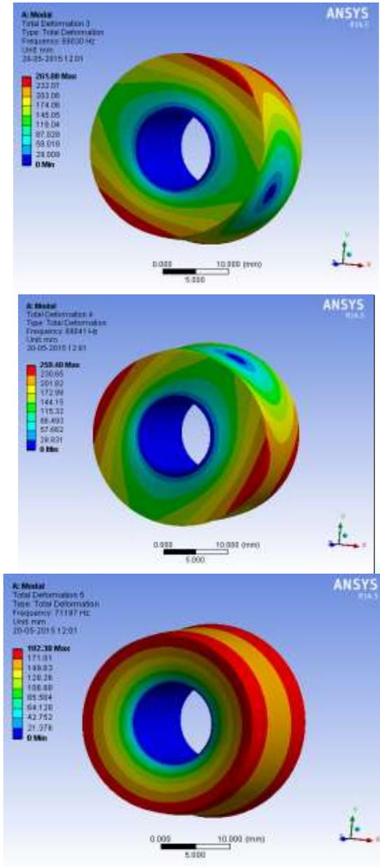
Fig 2.6 : Modal frequency at mode number 1,2,3,4,5, for stainless steel
