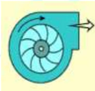
**Fig.1.** Backward curved centrifugal blower
