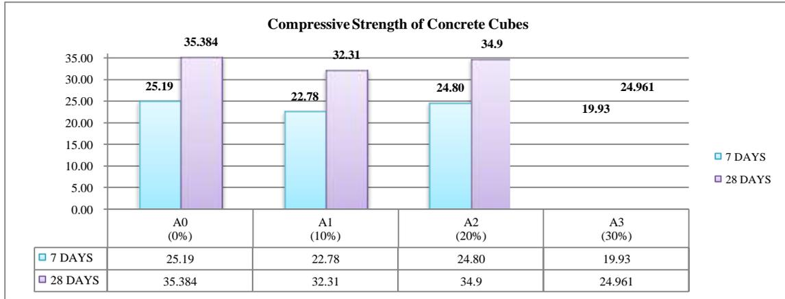
Fig. 3. Compressive strength of Concrete Cubes at 7 and 28 days
