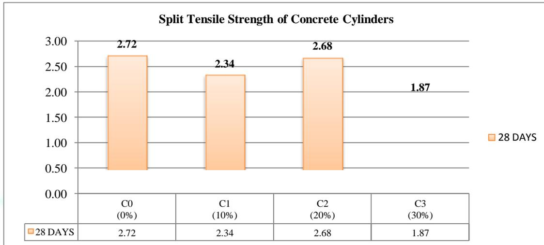
Fig. 5. Split tensile strength of Concrete Cylinders at 28 days
