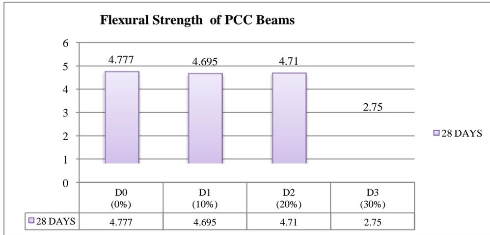
Fig. 6. Flexural Strength of Concrete Beams at 28 days
