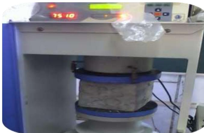
Fig. 1. Testing of Compressive Strength of Concrete Cubes
