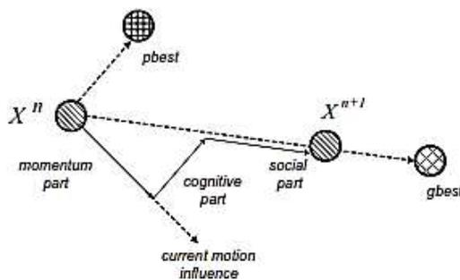
Fig. 3. Position updates in a PSO for a two dimensional parameter space.
