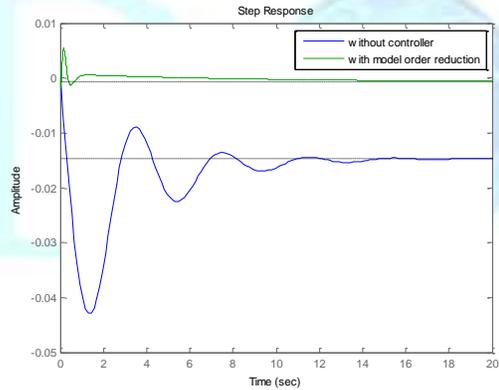
Fig.6. change in frequency due to step load (0.01p.u) change in area 1
