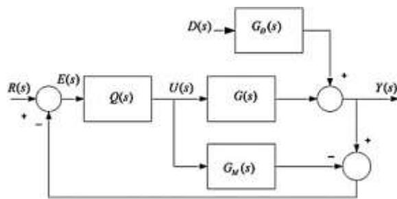
Fig1. Basic IMC structure.
