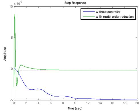
Fig.5. change in tie-line due to step load (0.01p.u) change in area 1
