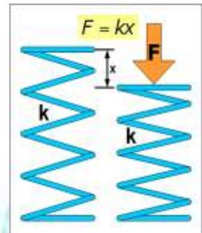
Figure 3. spring mechanics
