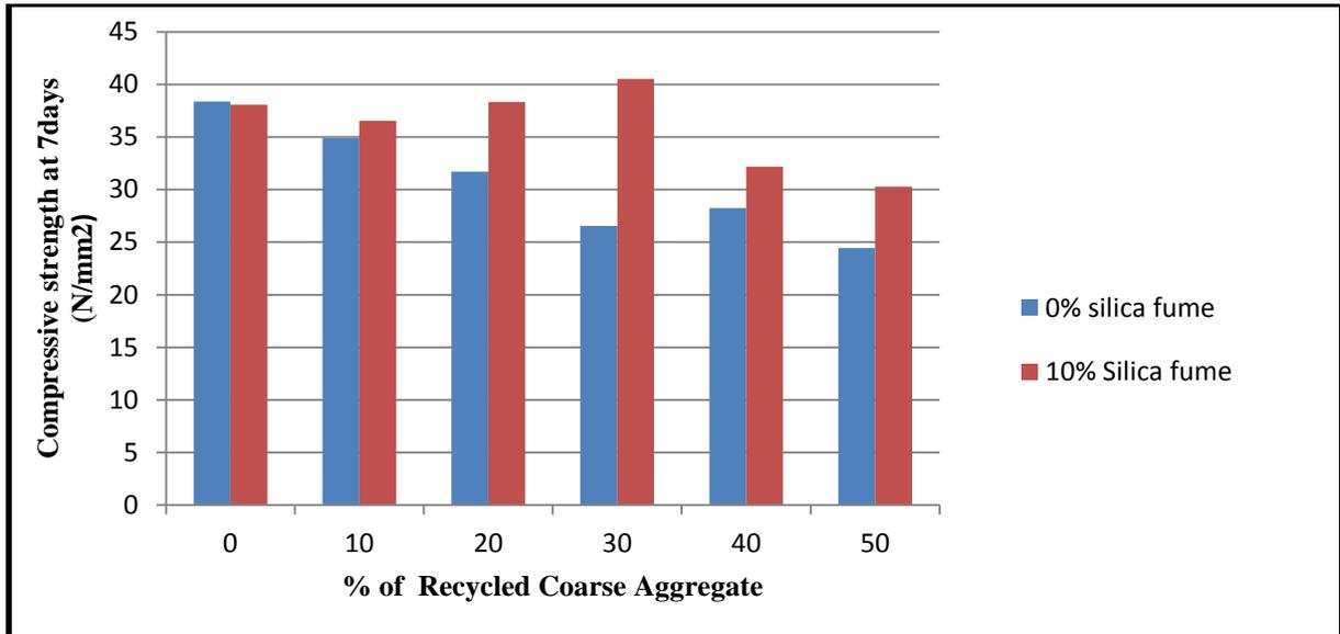
**Figure 3:** Effect of recycled coarse aggregate on compressive strength of concrete at 7days
