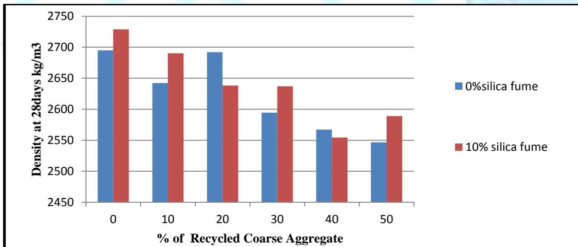
**Figure 1:** Effect of recycled coarse aggregate and silica fume on density of concrete
