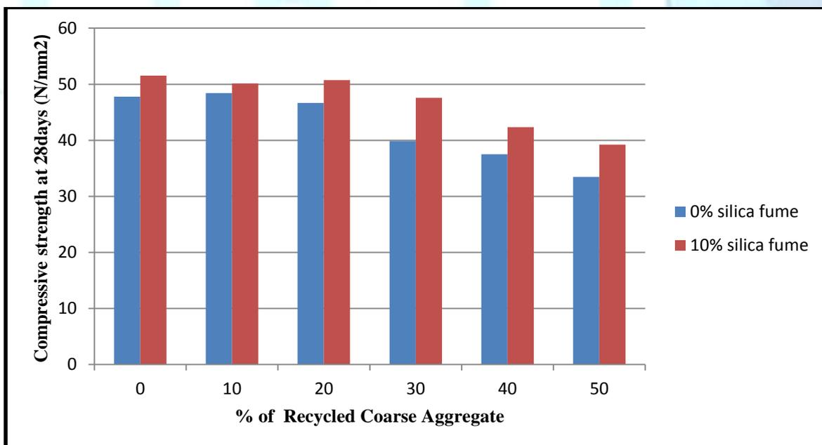
**Figure 4:** Effect of recycled coarse aggregate on compressive strength of concrete at 28days
