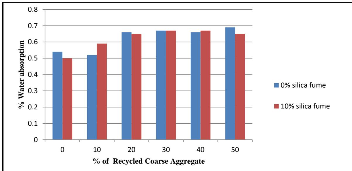
**Figure 2:** Effect of recycled coarse aggregate and silica fume on water absorption of concrete
