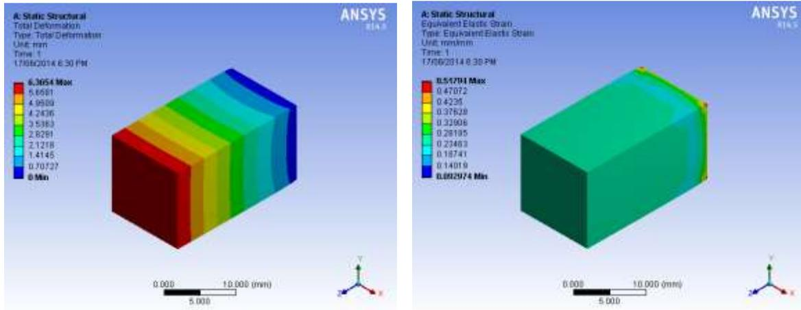
Fig 4.2 Total Deformation for pure epoxy Fig 4.3 Elastic strain for pure epoxy
