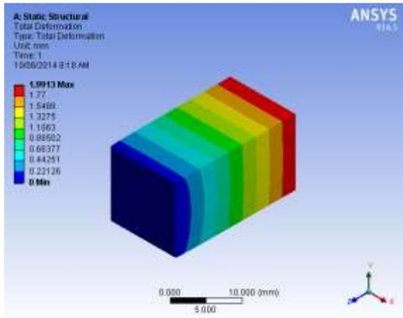
Fig 4.5 Total Deformation for 1%
