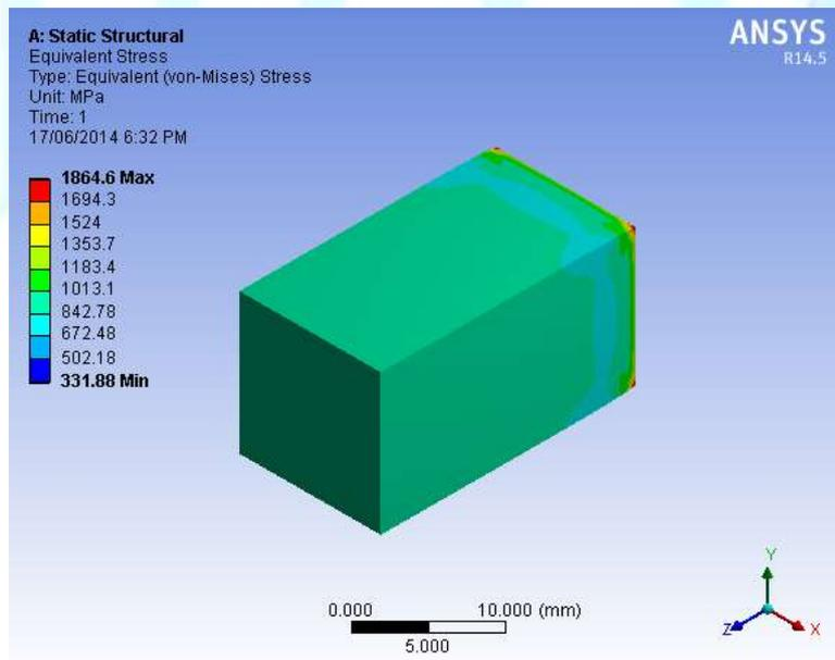
Fig 4.4 von misses stress for pure epoxy
