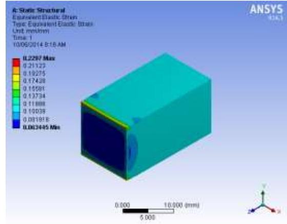
Fig4.9 Elastic Strain for 2%
