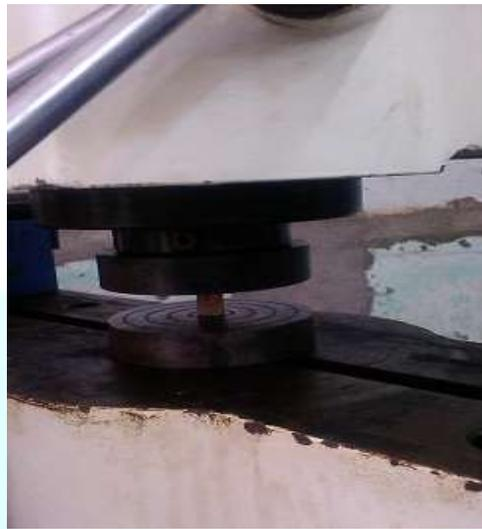
Fig 3.2 Specimen held at Universal testing machine for compression test.
