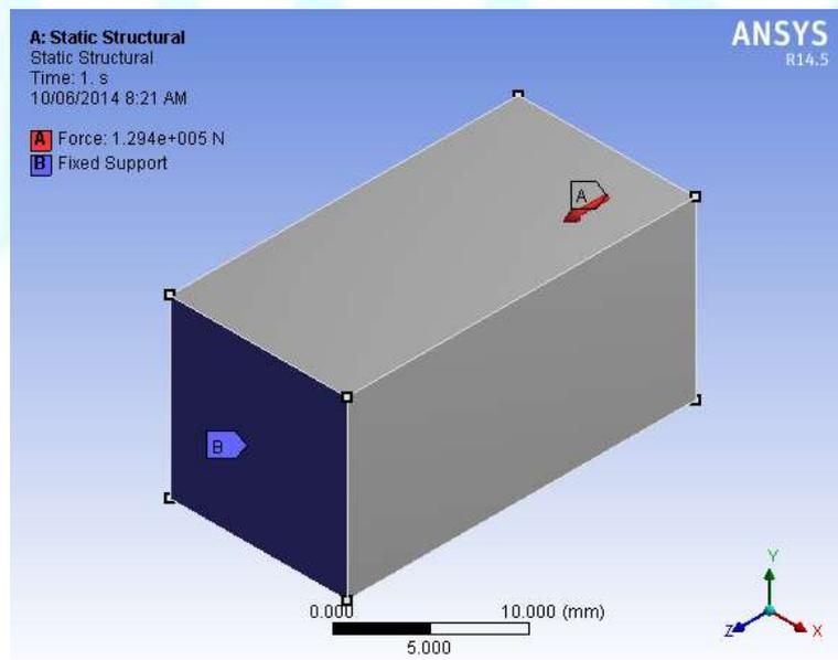
Fig 4.1 One end fixed and one end load applied
