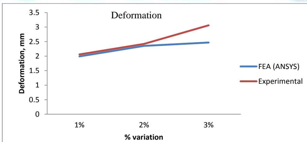
Fig 5.2 Comparison of FEA and experimental deformation for compressive test
