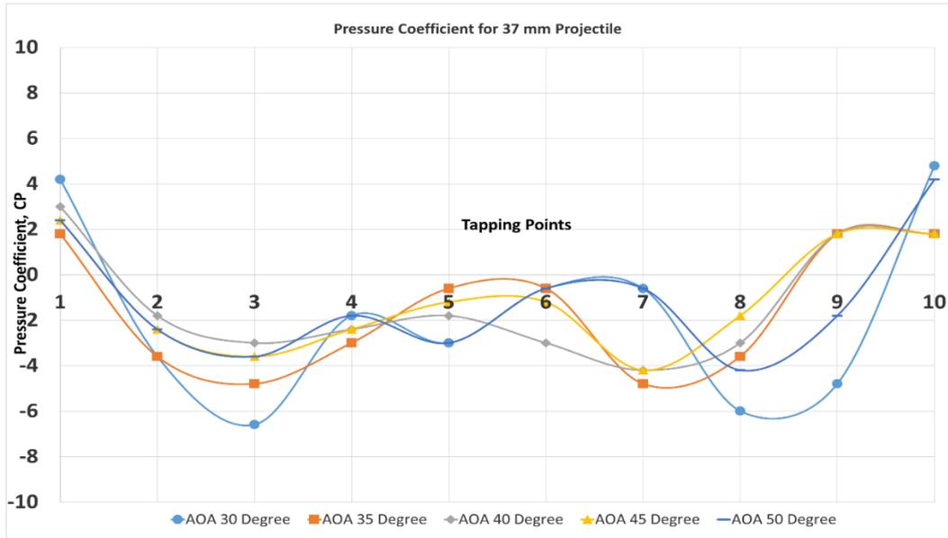
**Figure 12 :** Tapping Point Vs Pressure Coefficients for 37 mm Projectile.
