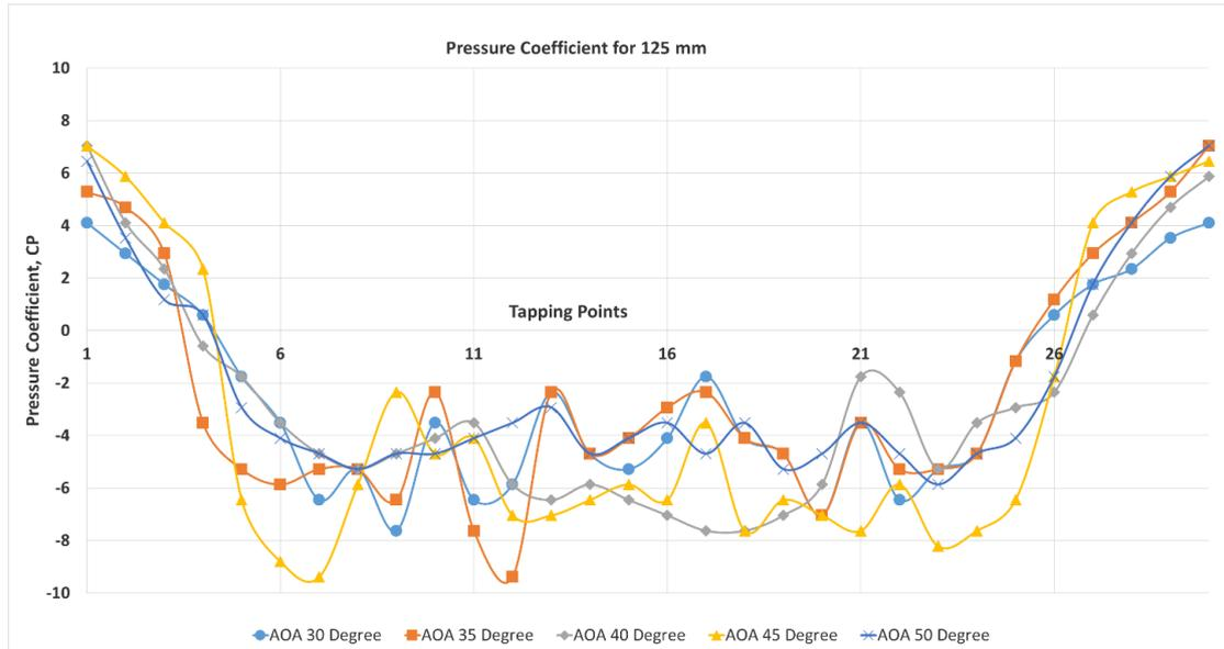
**Figure 14 : Tapping Point Vs Pressure Coefficients for 125 mm Projectile.**
