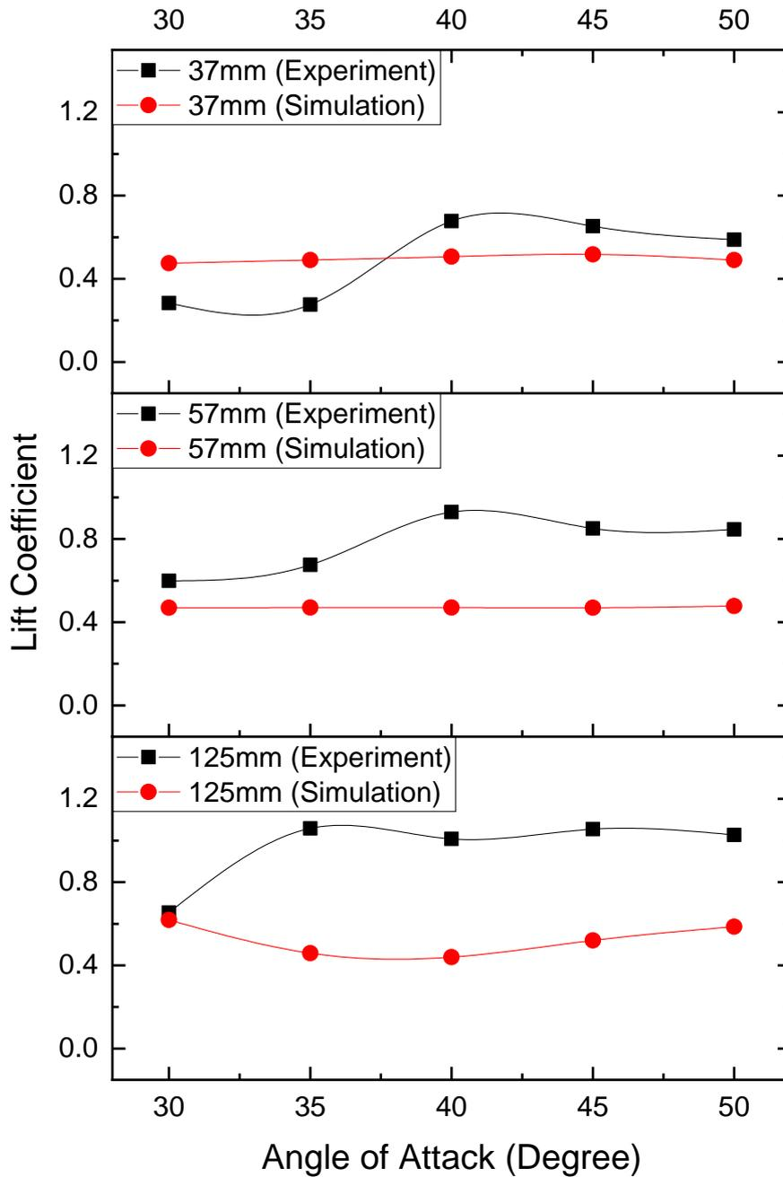
**Figure 11** : Angle of Attack vs Lift Coefficients.
