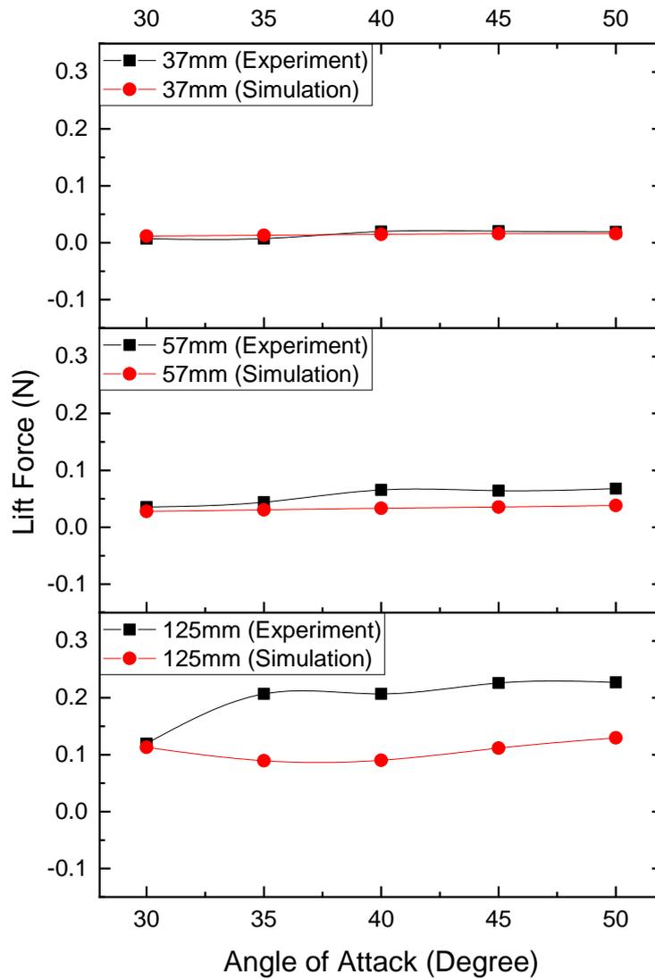
**Figure 9 :** Angle of Attack vs Lift Force.
