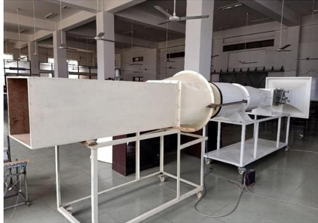
**Figure 5:** Open circuit subsonic wind tunnel.
