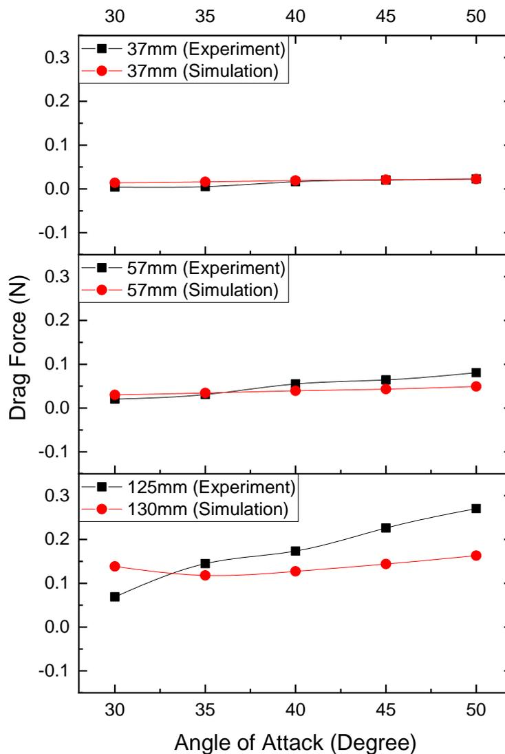
**Figure 8 : Angle of Attack Vs Drag Force.**
