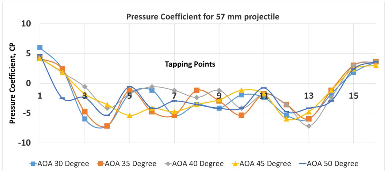
**Figure 13 :** Tapping Point Vs Pressure Coefficients for 57 mm Projectile.
