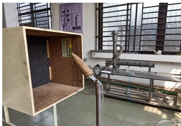
**Figure 6:** Test section with hollow projectile.
