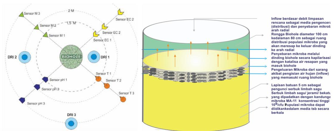
**Figure 2. Distribution Sensor Position & Biohole Structure**
