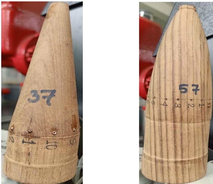
**Figure 1** : Dummy Model of existing 37 mm & 57 mm Projectile
