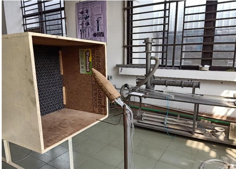
**Figure 4:** Experimental setup of projectile for measuring static pressure.
