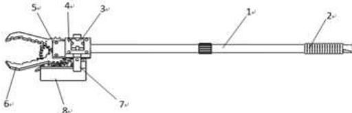
**Fig.1 Graphic model of the mechanism**
