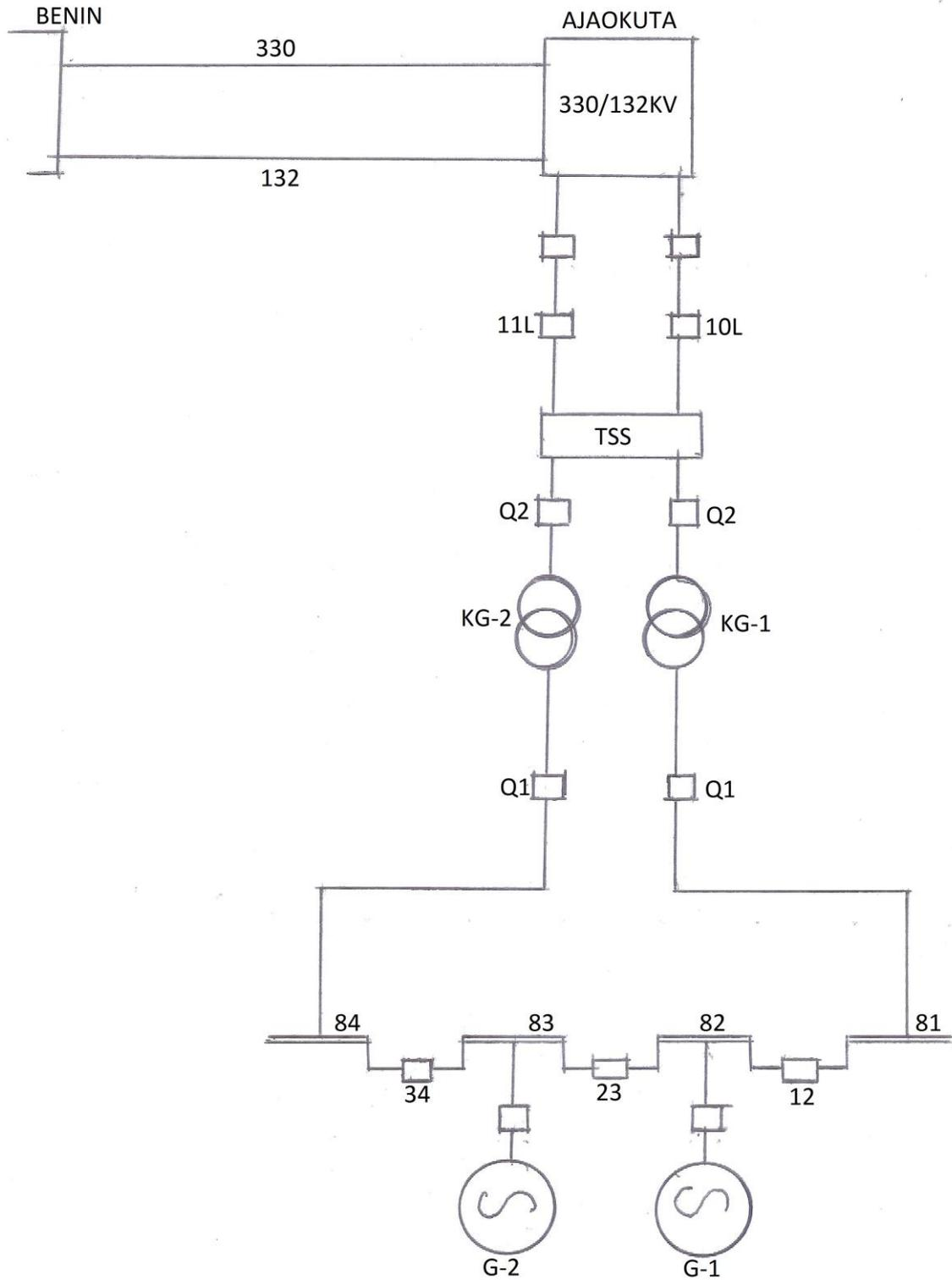
**FIG. 1 SYNCHRONIZATION BUSBAR AT TPP/TBS AJAOJUTA, NIGERIA**
