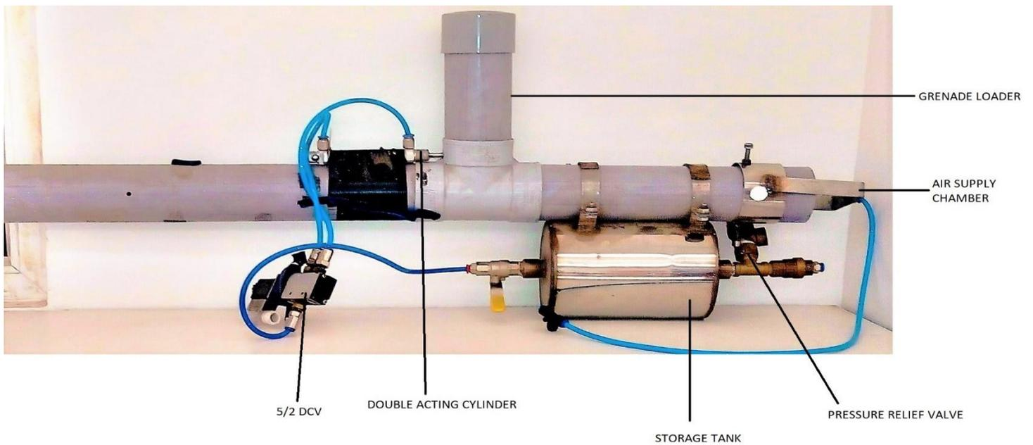
Figure 5 Assembled pneumatic launcher with storage tank
