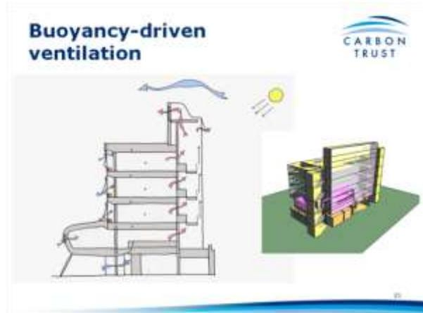
**Fig. 4** The inside and outside temperatures must be different
