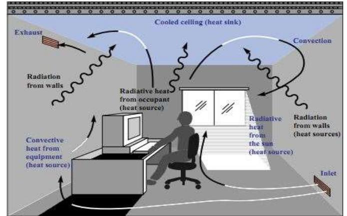
**Fig. 1** Explaninon of radiant coolong system in figure.
