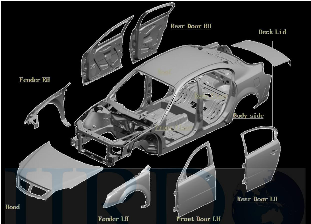
FIG. 1 AUTOMOBILE BODY THAT CAN STAMPED OR PUNCHED(Allen Bradley)
