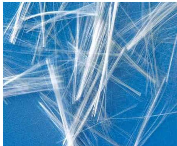
Figure 1-Glass Fibre
