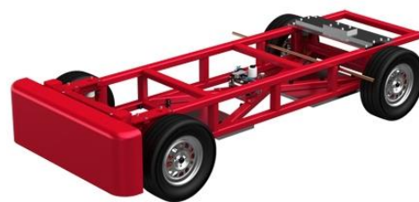
Fig.1.3. Frame Structure of a Fore Wheel Drive
