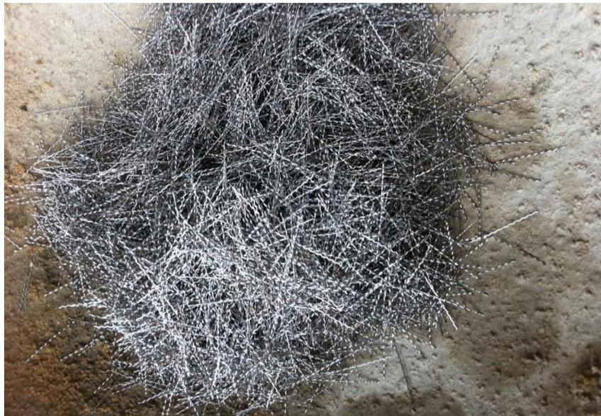
**Fig 1.1 Steel crimped fiber**
