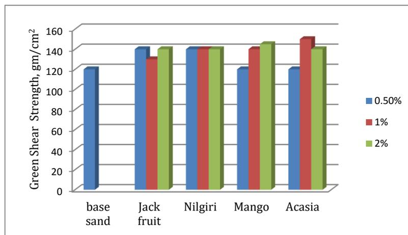
**Fig. 4** Effect of different % of Wood Additives on Green Shear strength, gm/cm<sup>2</sup>
