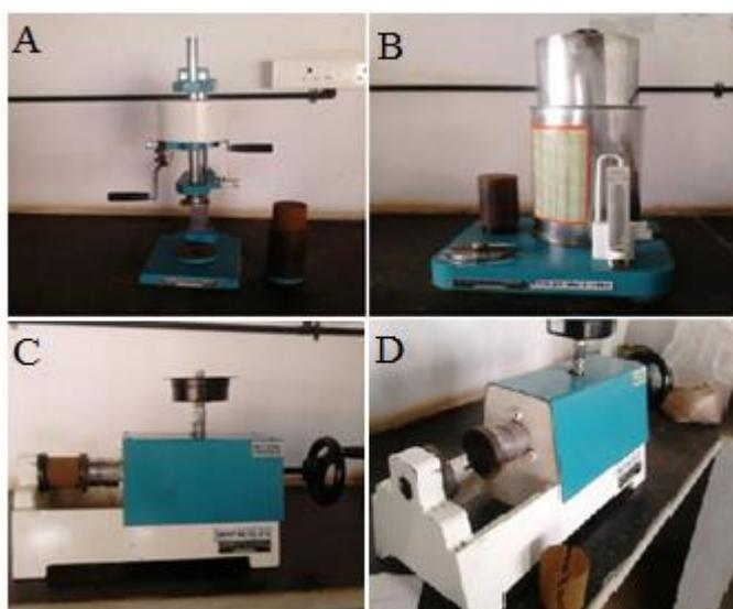
**Fig. 1** A) Sample preparation B) Permeability Tester C) Shear strength test setup D) Sand specimen after Shear test
