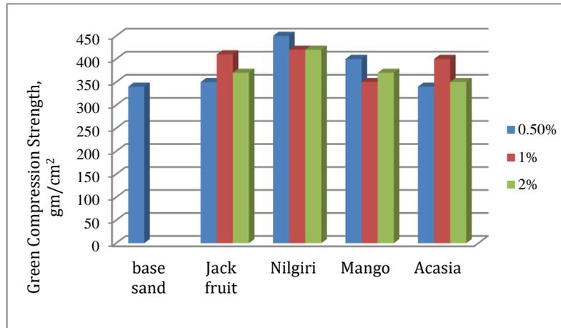
**Fig.3** Effect of different % of Wood Additives on Green Compression Strength, gm/cm<sup>2</sup>
