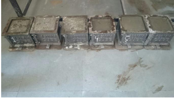
Fig. 2 After making the cube put it in to the immersion method of curing for 7 days and then the cube is tested.
