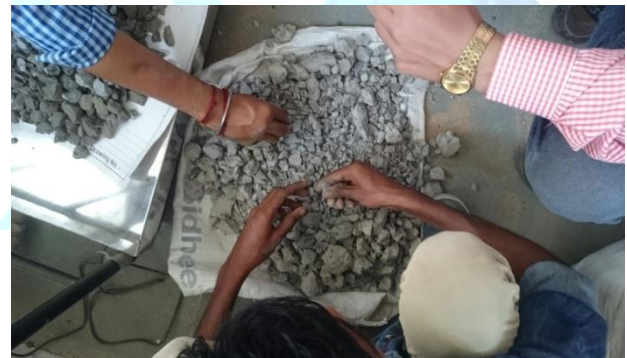
FIG.1 REMOVE THE CEMENT DUST ON AGGREGATE WITH HAND OR HAMMER
