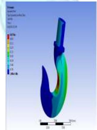
Fig 2:-Stress in triangular Hook
