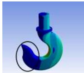
Fig 7:-Stress pattern in crane hook
