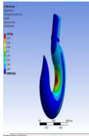
Fig 1:-Stress in Circular Hook
