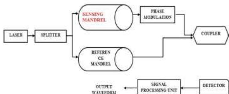
Fig 1. Block diagram of hydrophone
