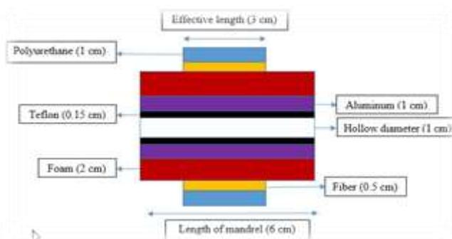
Fig 2. Proposed sectional view of mandrel
