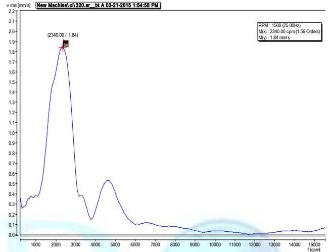
Fig. 5. RESPONSE OF CAST IRON
