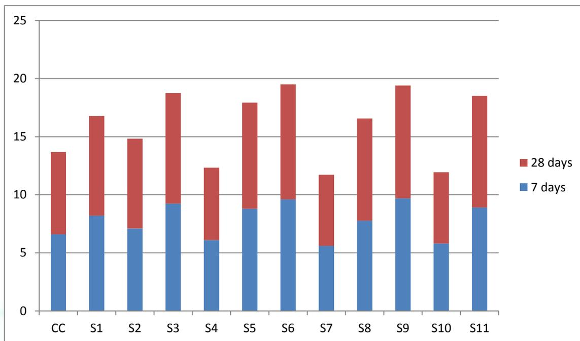
**Figure2.Graph result for Split tensile strength**
