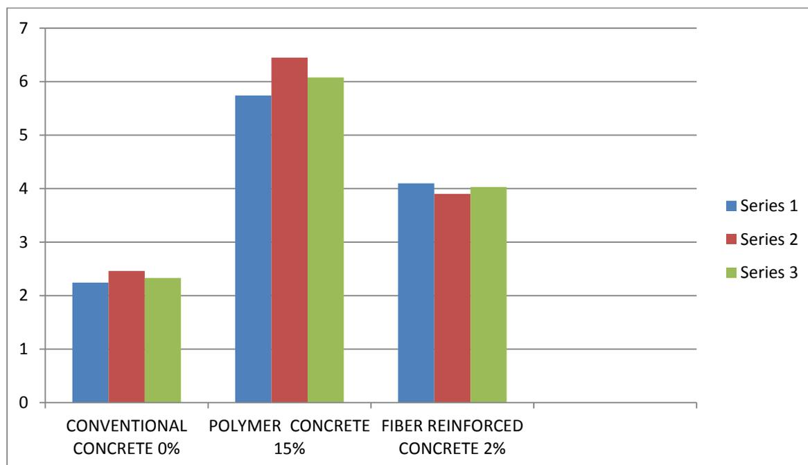
**Figure 7** Comparison of tensile strength results
