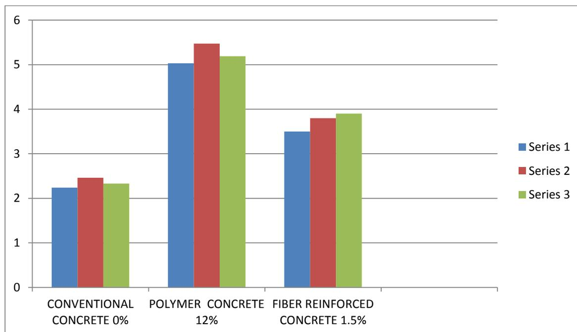
**Figure 6** Comparison of tensile strength results
