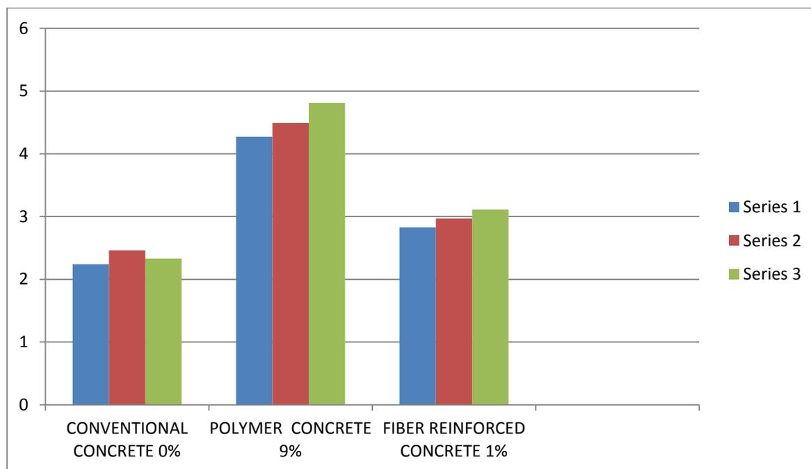
**Figure 5** Comparison of tensile strength results
