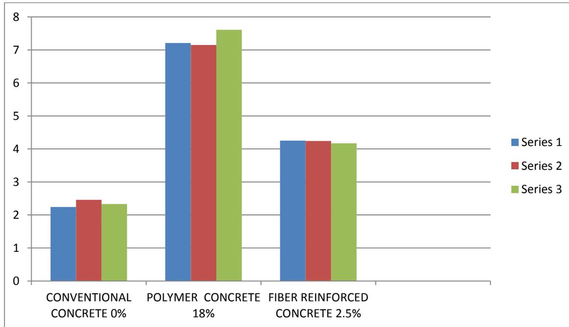
**Figure 8** Comparison of tensile strength results
