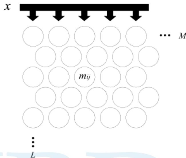
Fig. 1. Array of nodes scheme in a two-dimensional SOM grid.
