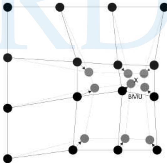
Fig. 2. Updating the BMU and its neighbours towards the input sample  $x$ . The solid and dashed lines correspond to the situation before and after updating, respectively.
