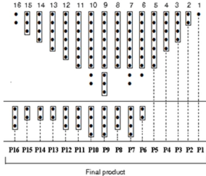
Fig.5. Dot Diagram of 8X8 multiplier
