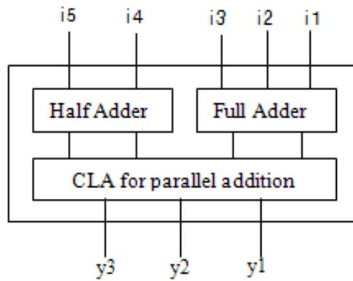
Fig.2. Block diagram of a 5-3 Compressor
