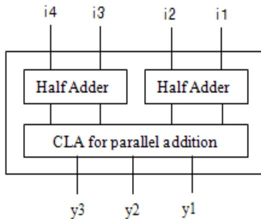
**Fig.1. Block diagram of a 4-3 Compressor**
