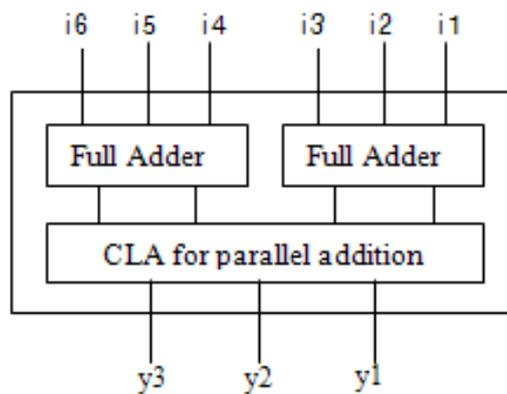
Fig.3. Block diagram of a 6-3 Compressor
