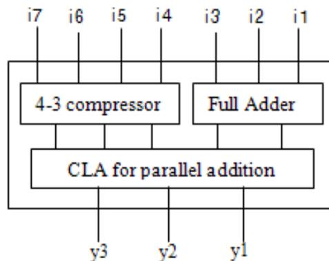
Fig.4. Block diagram of a 7-3 Compressor
