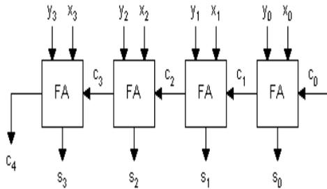
Fig.4 Ripple Carry Adder (RCA)
