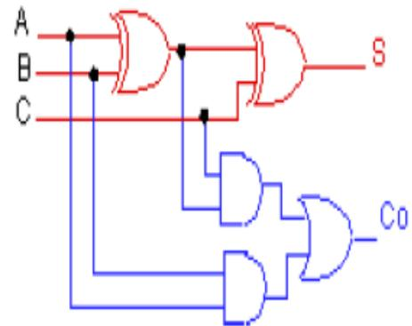
Fig.2 Full Adder Module
