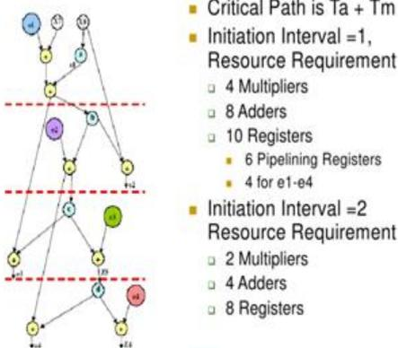
Fig.5 4 Stage Pipelining
