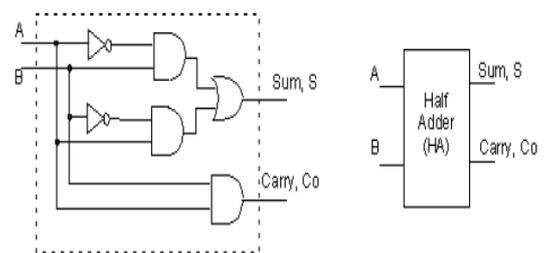
Fig.1 Half Adder Module
