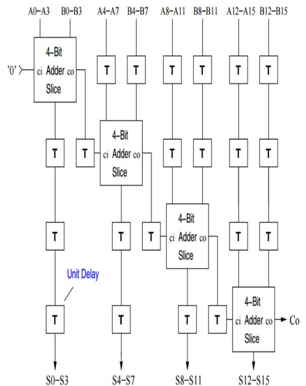
Fig.6 16 bit pipelined RCA adder
