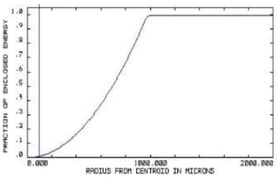
Fig. 7: Encircled energy on the PV cell.
