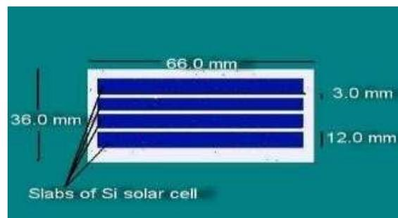
**Fig. 3: Solar Cell consists of four rectangular slab.**
