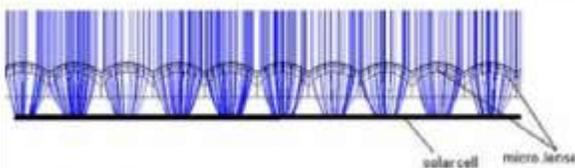
**Fig. 2: New design of micro-lenses concentrator**
