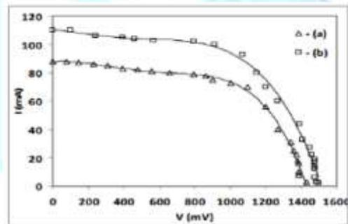
Fig. 5: V-I characteristics for PV Si cell without (a) and with (b) array micro-lens.
