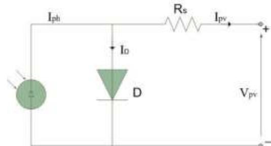
Fig. 4: Electrical diagram represent I-V characteristic measurements circuit.
