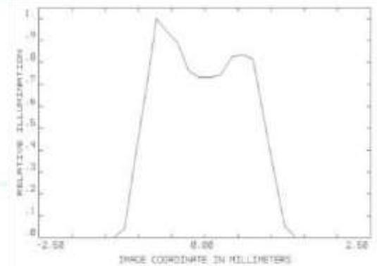
Fig. 6 : Illumination distribution on the PV cell slap.
