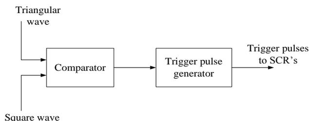
Fig – 2 Block diagram of SPWM
