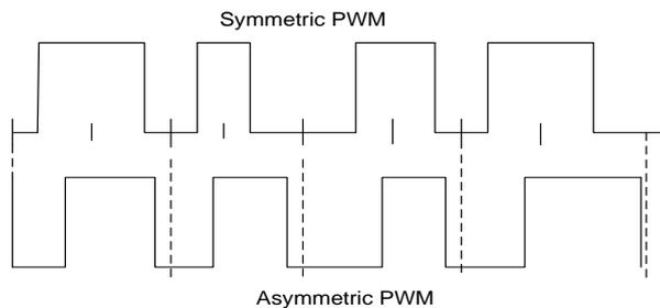
Fig 1 – Different types of PWM signals
