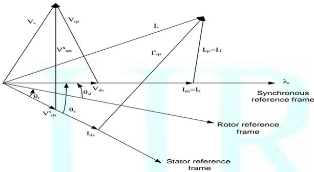
Fig -4 Phasor diagram of Induction machine
