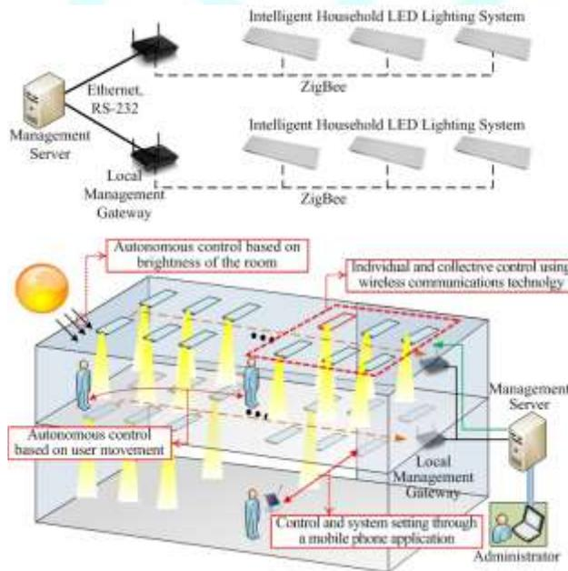
Fig.3 The wireless sensor arrangement and the overview of the system.
