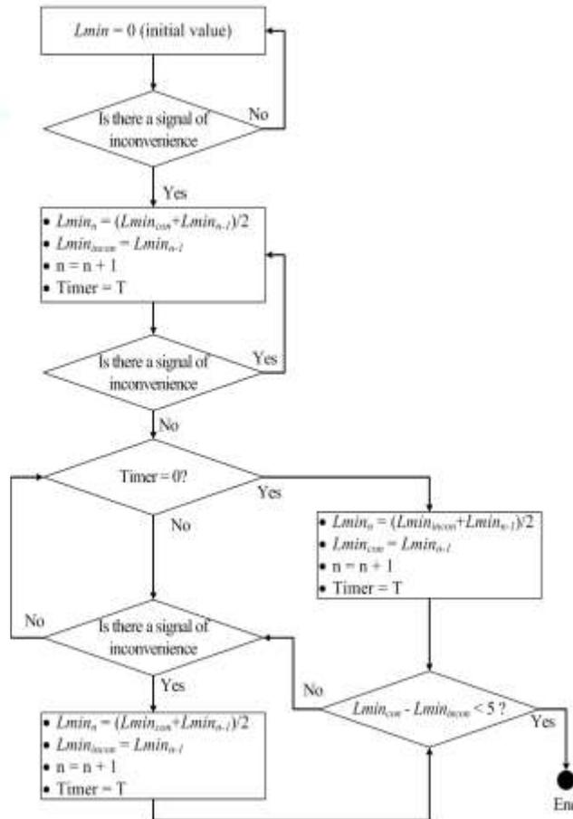
Fig.4 The minimum light intensity control flow chart.
