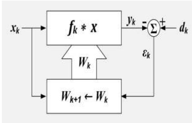
Adaptive Filter. k = sample number, x = reference input, X = set of recent values of x, d = desired input, W = set of filter coefficients, ε = error output, f = filter impulse response, \* = convolution, Σ = summation, upper box=linear filter, lower box=adaption algorithm
