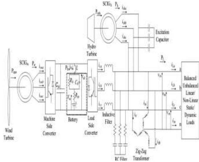
Fig1.Schematic diagram of wind hydro hybrid system
