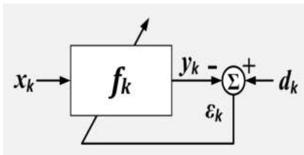
Adaptive Filter, compact representation. k = sample number, x = reference input, d = desired input, ε = error output, f = filter impulse response, Σ = summation, box=linear filter and adaption algorithm.
