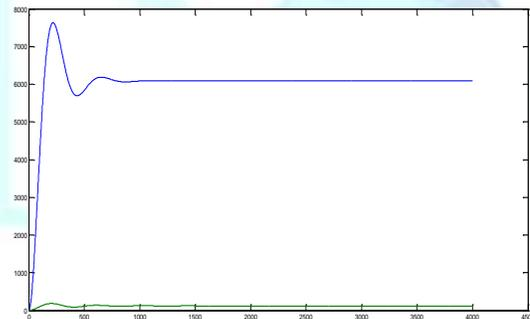
Fig3. Active and reactive power of wind turbine
