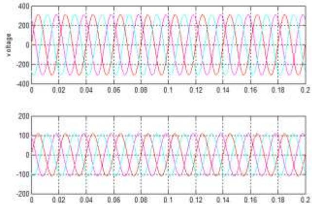
1. Input Voltage and current waveforms of wind turbine, V=310v, I=120A
