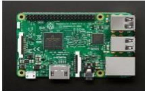
Fig. 2 Raspberry Pi 3 Model B+
