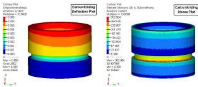
**Fig-5.9:** Deflection and Stress Plot (Cup without Carbonitriding)
