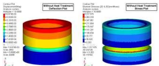
**Fig-5.8:** Deflection and Stress Plot (Cup without Heat Treatment)
