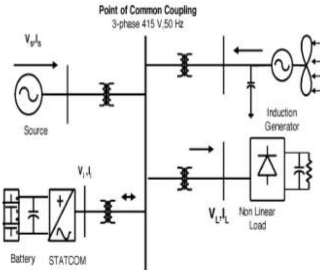
Fig. 1. Schematic diagram of micro-wind generator with battery storage for critical load application.
