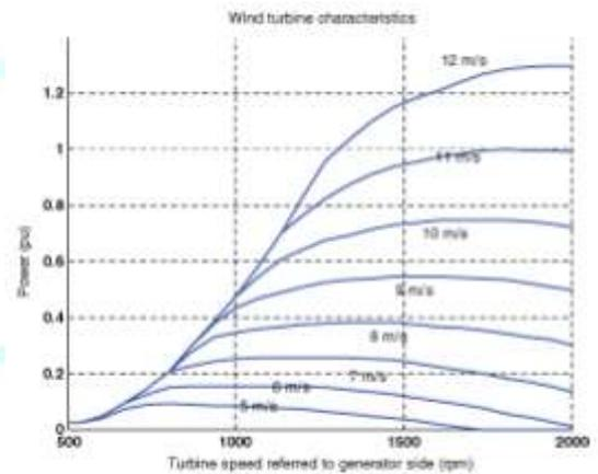
Fig. 2. Power-speed characteristic of turbine
