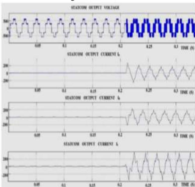
Figure 7. STATCOM voltage and current  $I_a, I_b, I_c$
