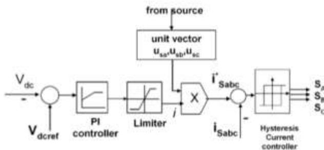
Fig. 5. Control scheme for switching the inverter circuit.
