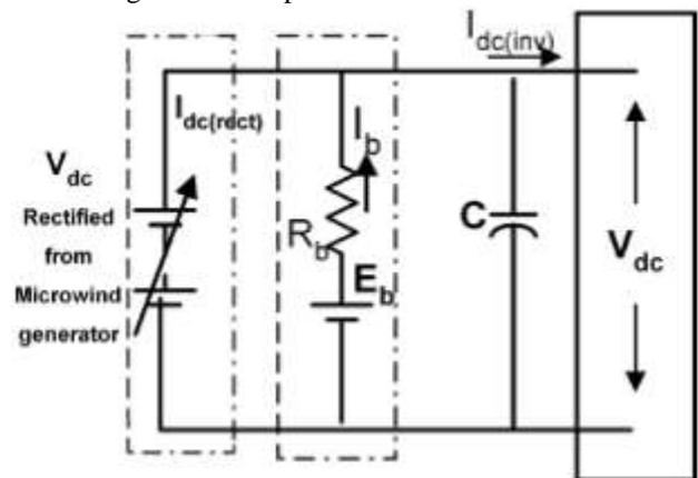
Fig. 3. Dc link for battery storage and micro-wind generator.
