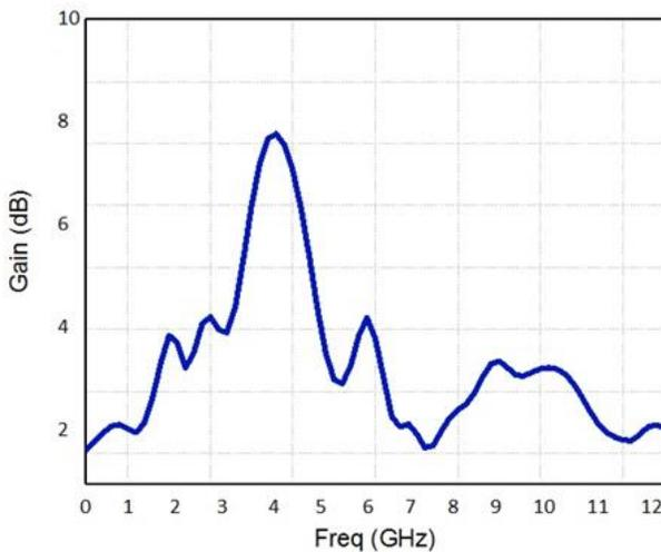
**Figure 7.** Proposed dual band antenna gain
