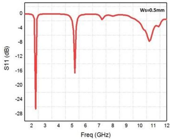
**Figure 5.2.** Effect of width of slot (*Ws*) on the result of *S11*
