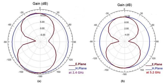
**Figure 5.** Radiation pattern at double frequencies (a) 2.4 GHz (b) 5.2 GHz
