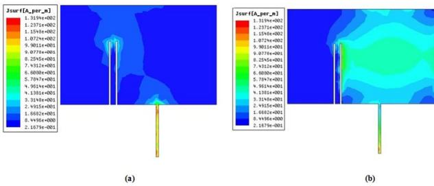
**Figure 6.** Current concentration at (a) 2.4 GHz(b) 5.2 GHz
