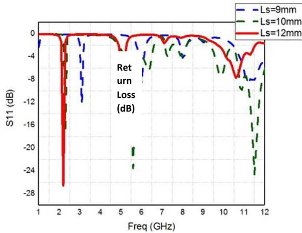
**Figure 3.** Effect of length of slot (Ls) on S11
