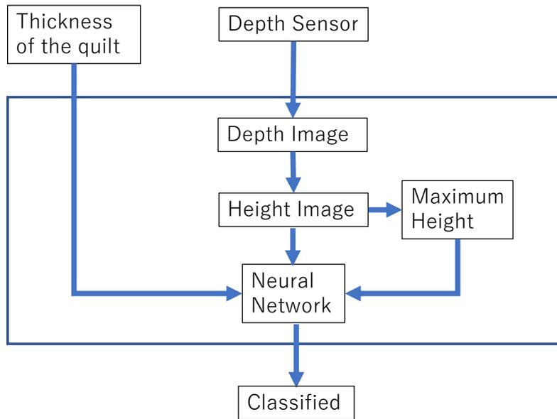
Fig. 2. Schematic diagram of the awakening detection system.
