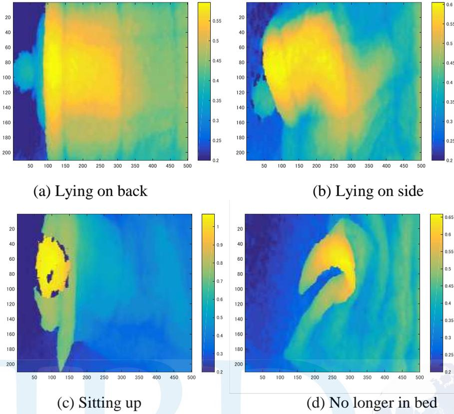
Fig. 6. Examples of height data for the four cases. The subject is covered by a thick quilt. One pixel is equal to 4.5 mm, and the color bars are in meters.
