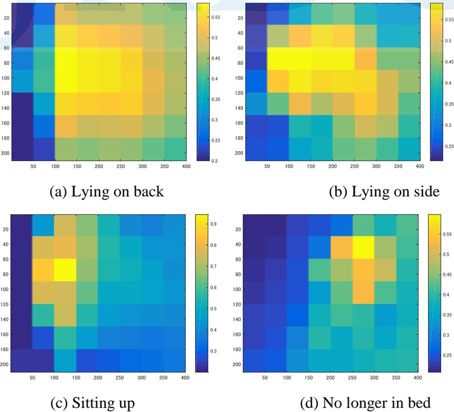
Fig. 7. Examples of height data for the four cases at a low resolution of  $7 \times 8$  pixels. The subject is covered by a thick quilt. The color bars are in meters.
