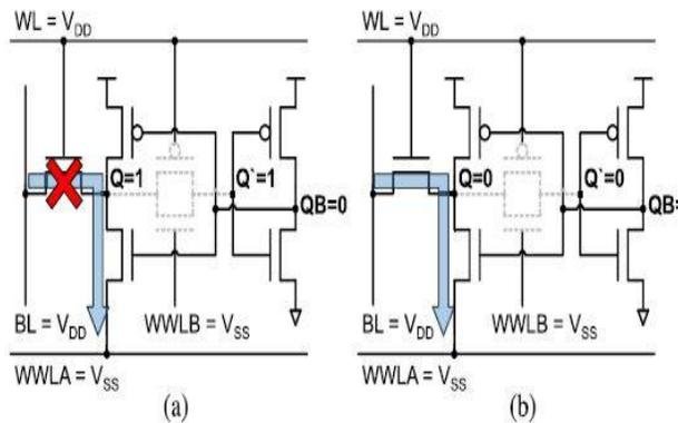
Fig.4. (a) Read “1” and (b) “0” operations of 7T SRAM cell.
