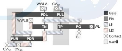
Fig.2. Single cell layout of existing 7T SRAM cell
