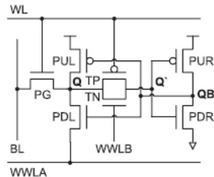
Fig.1. Schematic of the existing 7T SRAM cell.
