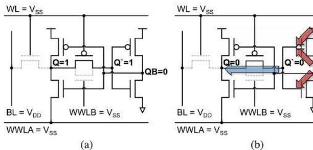
Fig.3. (a) Storing “1” data and (b) storing “0” data in hold mode.
