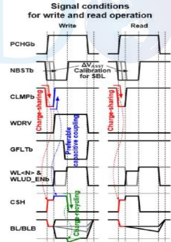
Fig.9. Timing diagram of proposed charge-recycling assist technique
