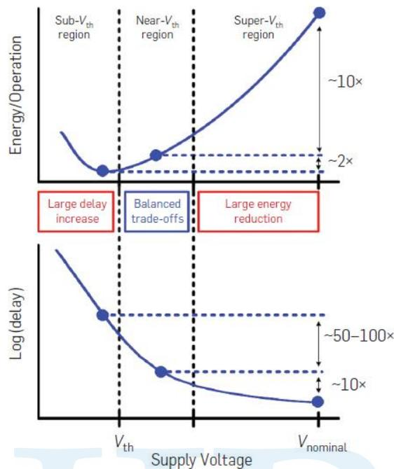
Fig.10. Energy and delay in different supply voltage operating regions.
