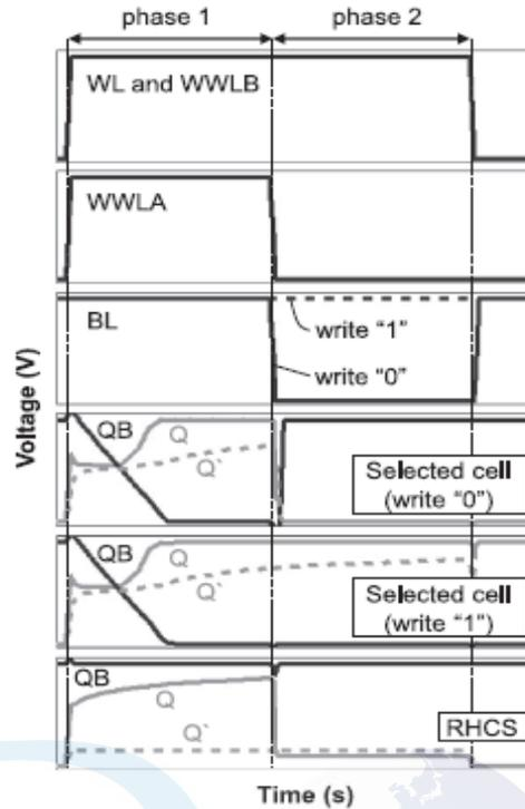
Fig.7. Waveforms of the write operation of the existing 7T SRAM cell.
