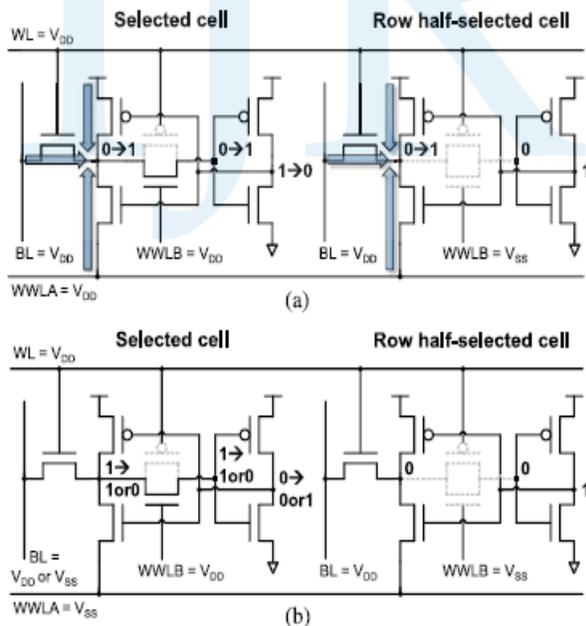
Fig.6. (a) Phase 1 and (b) phase 2 of the write operation of 7T SRAM cell.
