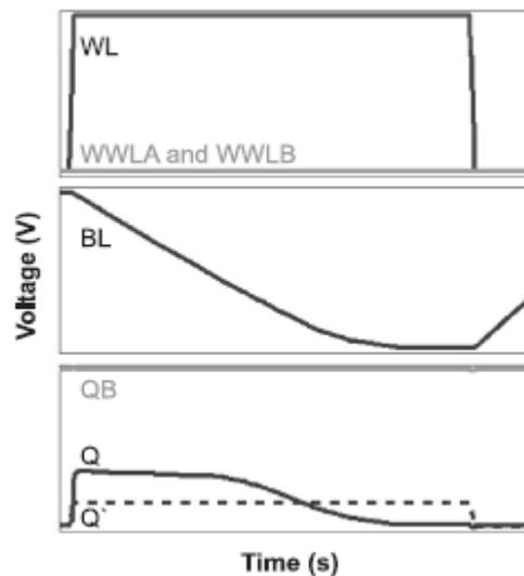
Fig. 5. Waveforms of the read operation in the existing 7T SRAM cell.
