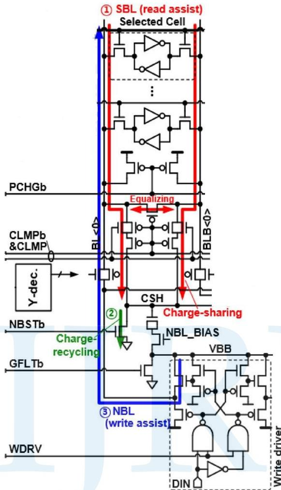
Fig.8. Schematic of proposed charge-recycling assist technique
