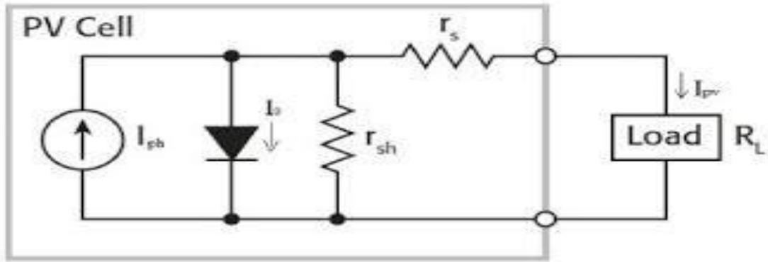
Fig:1 Equivalent circuit of PV cell: one diode ([https://www.researchgate.net/figure/284810777\\_fig\\_2Single-diode-equivalent-circuit-model-of-solar-cell](https://www.researchgate.net/figure/284810777_fig_2Single-diode-equivalent-circuit-model-of-solar-cell).)
