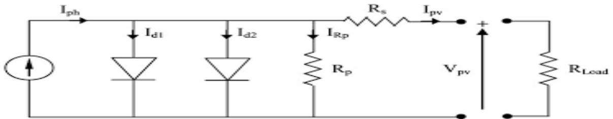
Fig:2 Equivalent circuit of PV cell: Two diodes ([http://file.scirp.org/Html/1-6401030\\_3323.htm](http://file.scirp.org/Html/1-6401030_3323.htm).)
