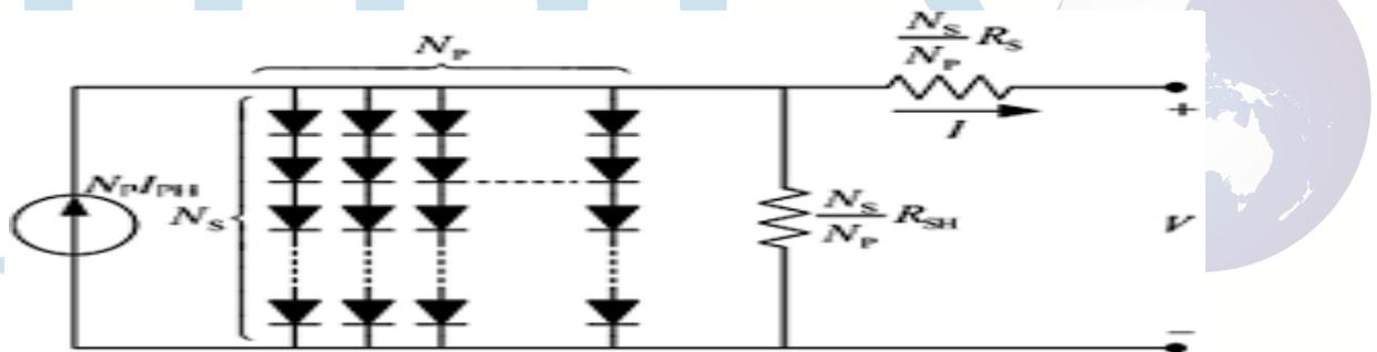
Fig:3 Equivalent circuit of PV cell: Multiple diodes (<http://link.springer.com/content/pdf/10.1186%2Fs40068-015-0047-9.pdf>.)
