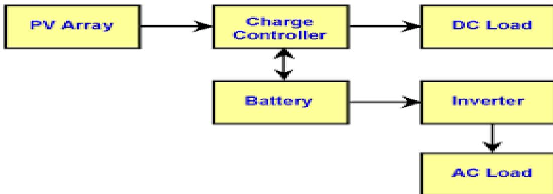
Fig:4 Block diagram of PV system. ([http://www.fsec.ucf.edu/en/consumer/solar\\_electricity/basics/types\\_of\\_pv.htm](http://www.fsec.ucf.edu/en/consumer/solar_electricity/basics/types_of_pv.htm).)
