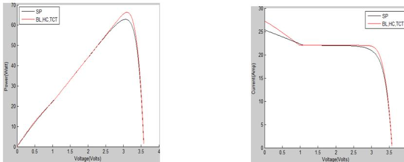
Fig.7.6 : P-V and I-V Characteristics for randomly shaded pattern-III
