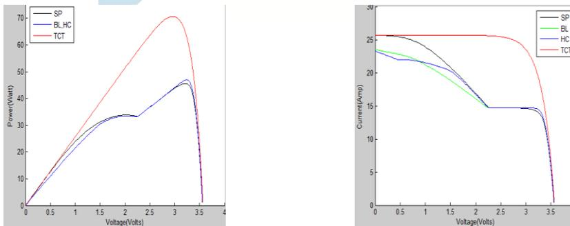
Fig.7.5 : P-V and I-V Characteristics for randomly shaded pattern-II
