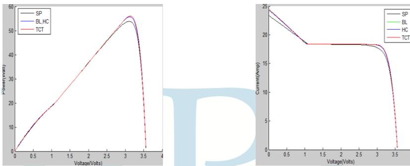
Fig.7.4 : P-V and I-V Characteristics for randomly shaded pattern-I
