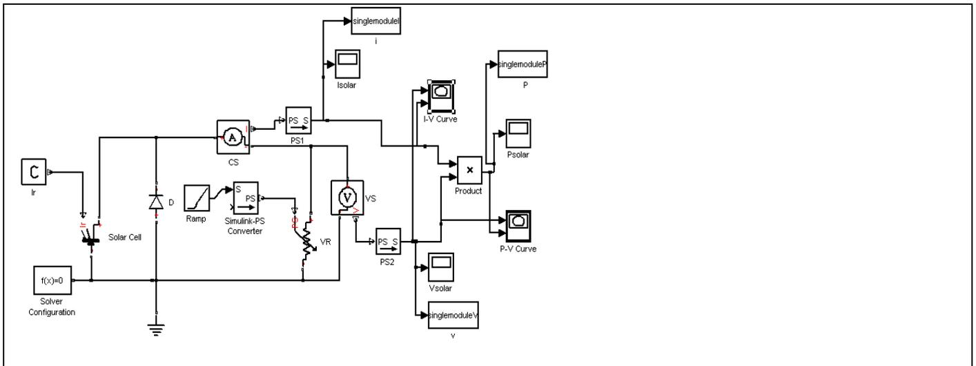
Fig.2 : Model of single solar cell in MATLAB/SIMULINK
